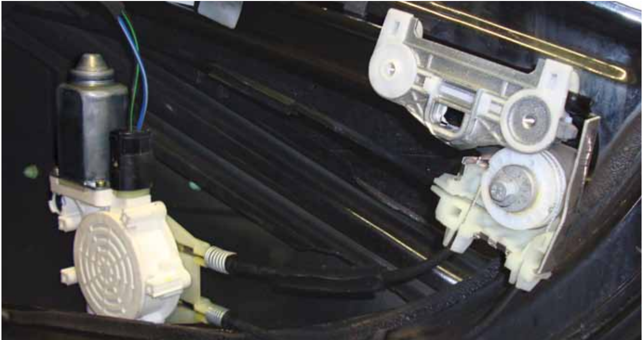
This 3-Series has cable-driven window regulators. They're lighter and simpler to service than the scissors-type, but more sensitive to binding glass.
