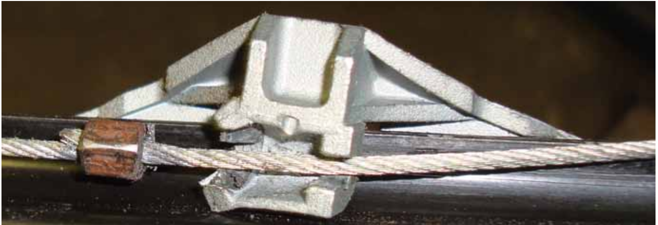
Damage such as this crack will raise havoc with power window operation.
