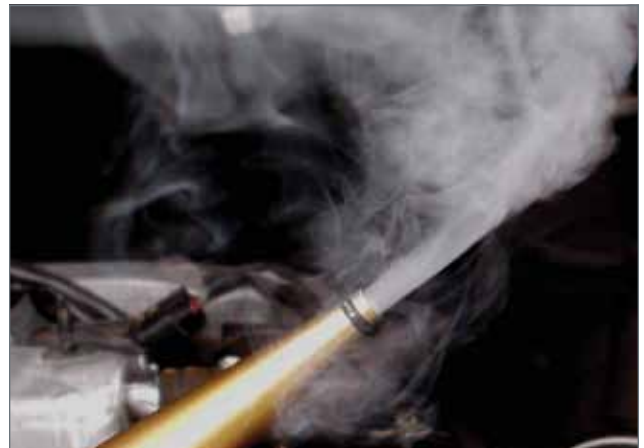
Figure 8: Using your smoke machine is an easy way to find intake leaks.
