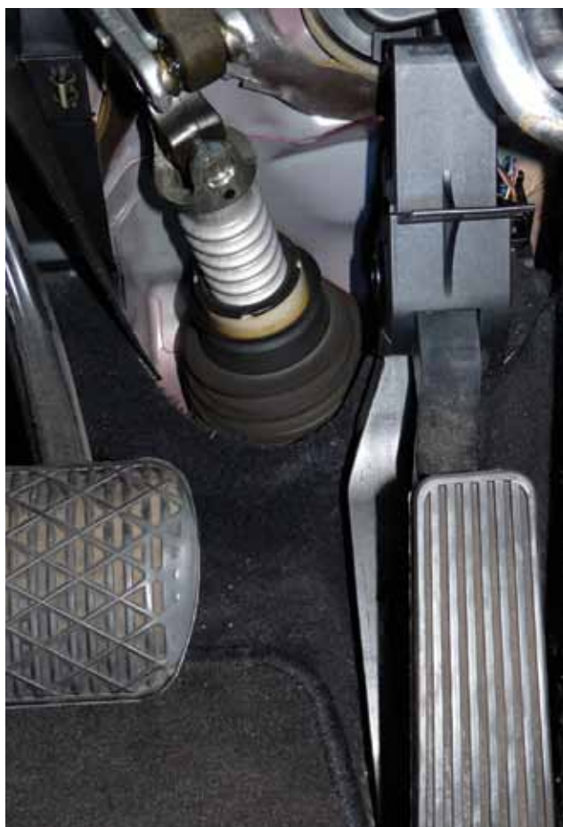
If the Electronic Accelerator sensor has any corrosion issues, your testing may indicate that it is out of specifications.
