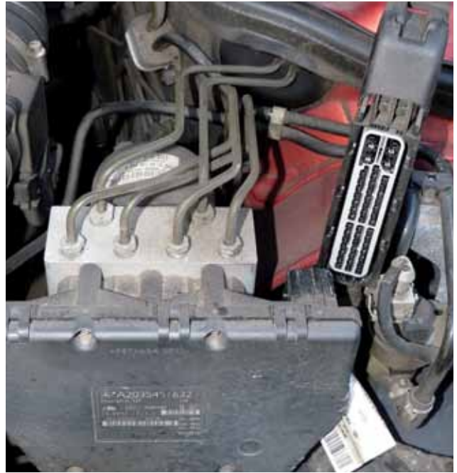
Here is an example of an ESP Control Unit on a 2002 C-class. Aftermarket ignition components may not be as protected against causing high electromagnetic field (EMF) possibly damaging the ESP Control Units that are mounted on the hydraulic units.
