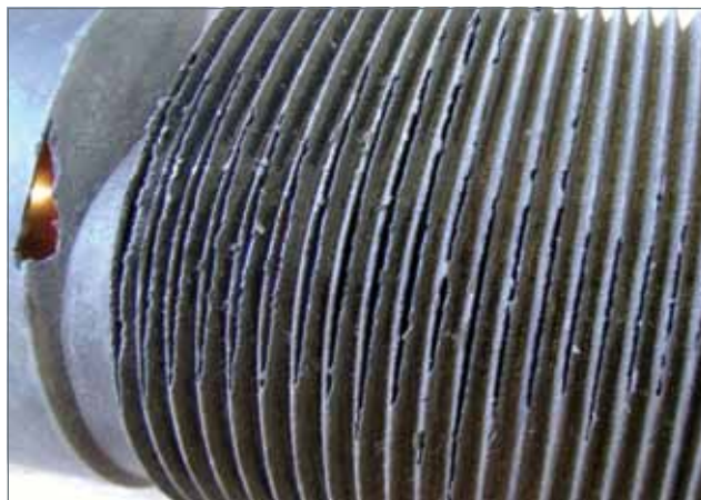
When the duct downstream of the Air Mass Sensor fails like this, it admits “false air.”
