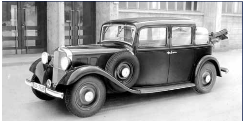
Mercedes-Benz introduced the world's first passenger-car diesel in 1936, the 260D.
