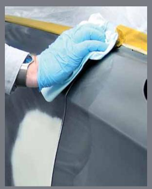
Obviously, paint will not stick to dirt or oil-based contaminants. Before and after sanding and between undercoats and topcoats, clean the surface with wax and grease remover.
