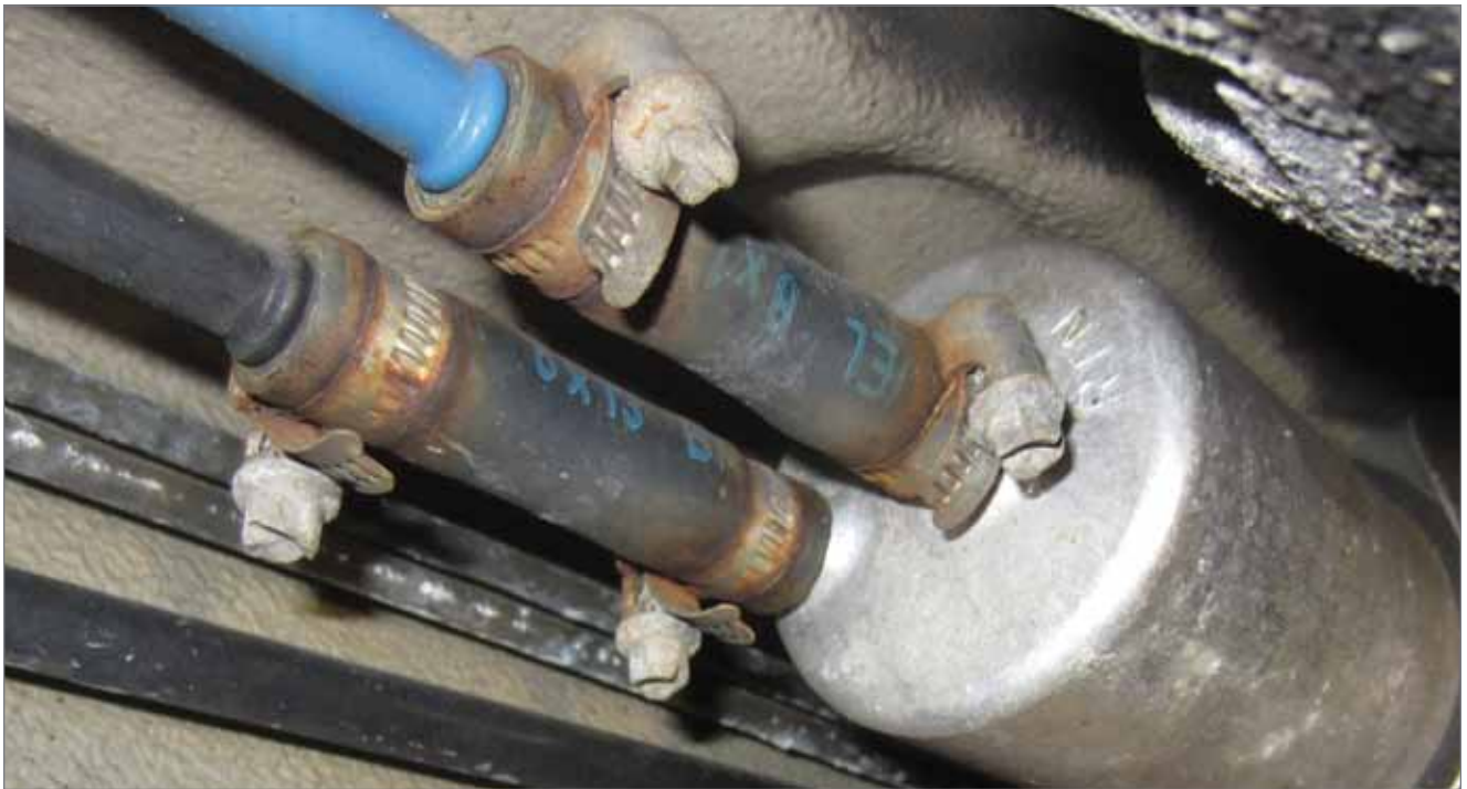
This is where the fuel filter is located on the E46. The fuel volume gauge is hooked up on the left (pump) side of the filter, not only because it is easier, but because it will also give us a more direct reading.
