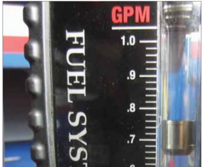
Here the fuel pump is apparently running strong with a fuel volume above specification.
