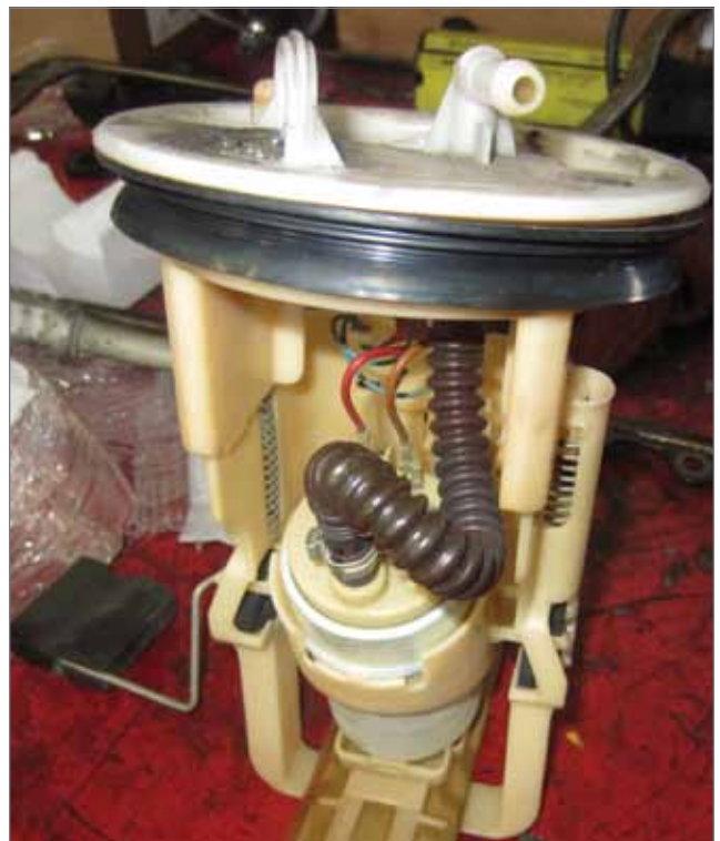
The OE BMW fuel pump assembly including the sending unit, made by VDO.
