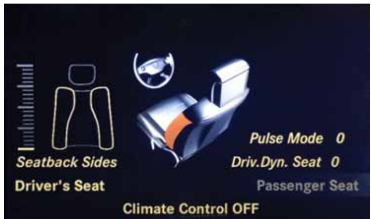
The Dynamic Seat function uses steering sensor input to instantly inflate the side cushions in tight turns to keep your body more stable.
