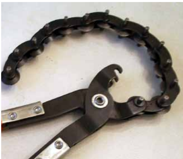
If you want to do some research into what's killing pumps among your customers, you can use an exhaust pipe cutter to slice through the aluminum housing and pull out the internal components. It's easy and interesting.
