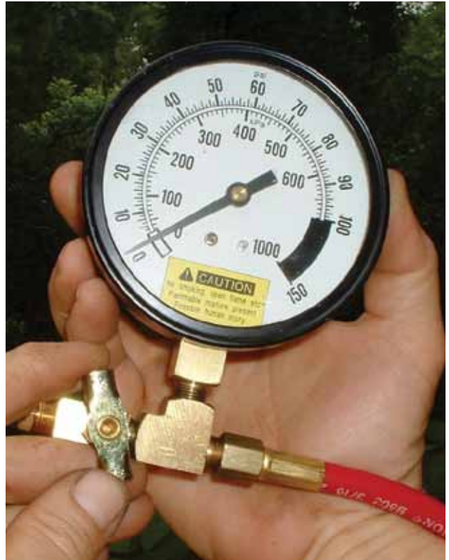
Good pressure doesn't necessarily mean sufficient volume. In some cases, just opening your gauge valve will kill the engine. Better do a volume test.
