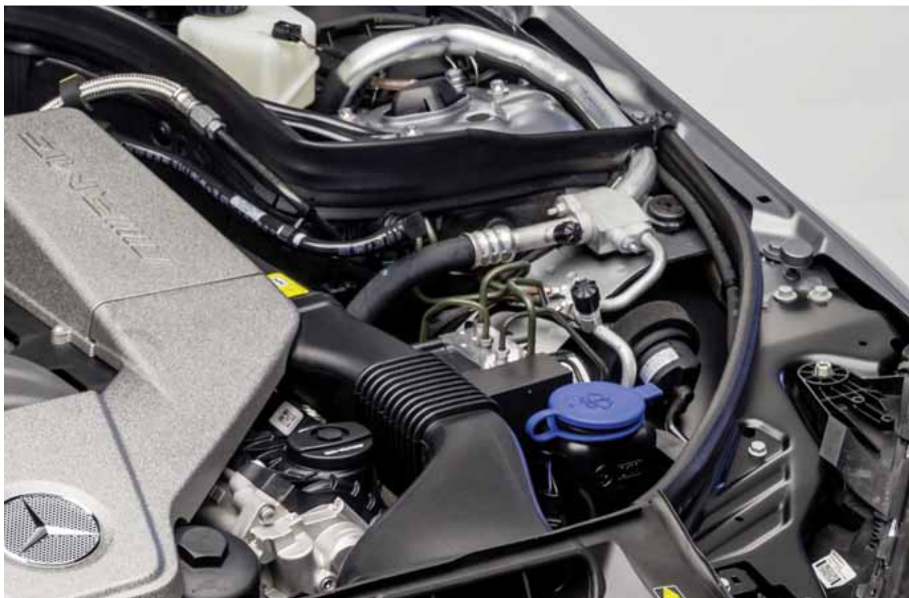
The AMG's A/C service ports are visible on the right. While not compatible with those for R-134a, they don't look that much different, and a retrofit can easily be made.
