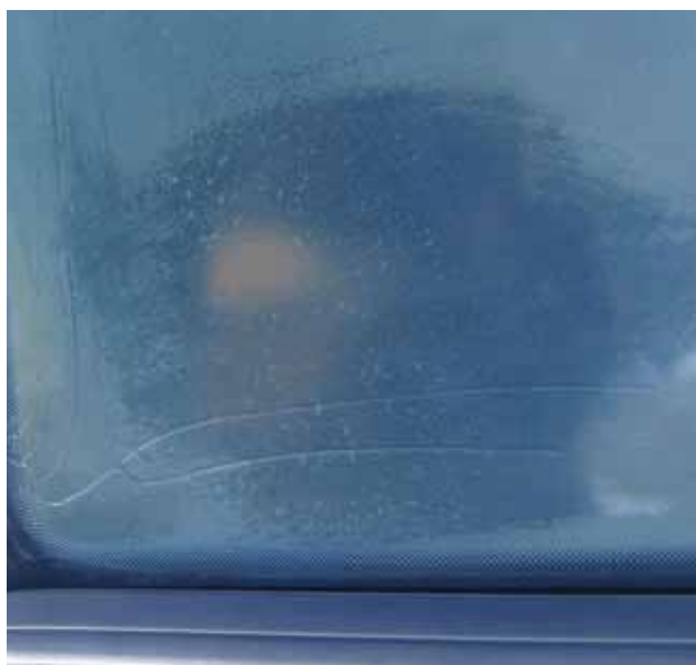
The hydrogen fluoride gas that's produced when "twelve thirty-four" burns in the engine compartment quickly infiltrates the cabin. It's so corrosive it etched this test car's windows to the point of opacity. This photo is from UBA, the German Federal Environment Agency.
