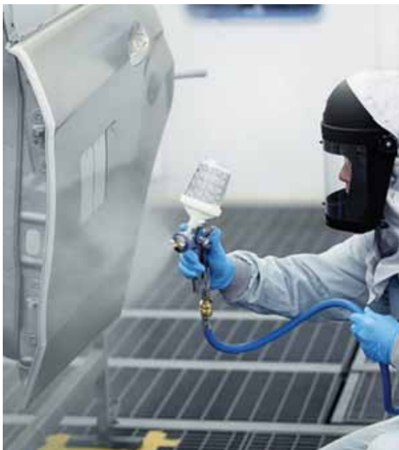
Color test panels are absolutely critical to match both color and gloss level to the vehicle being painted. Prepare several test panels, each featuring different mixing ratios of matting agent and clearcoat, and different wet/dry spraying methods.
