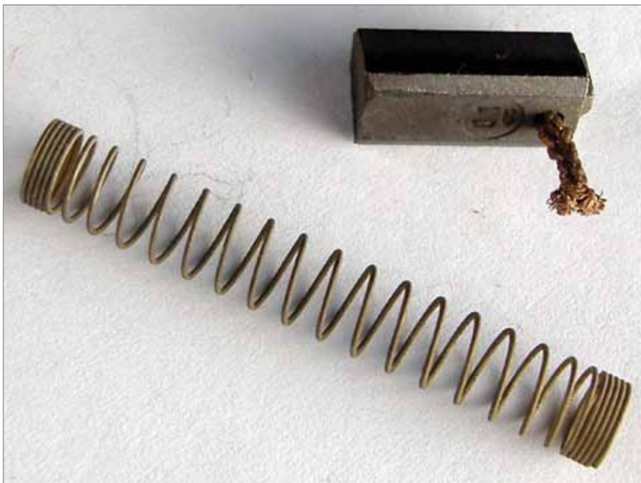
Excessive oscillations of the brushes can cause their leads to break from fatigue. If the springs are grounded, they'll complete the circuit, but not for long. In later versions, the brush holders are all nylon, so there's no path to ground through them.
