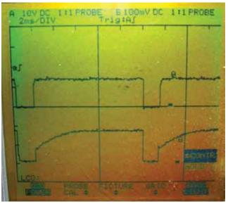
One way to analyze VANOS solenoid operation is to monitor the current pattern of an activated solenoid. Here, the intake cam advance solenoid has been activated by accelerating the engine. Notice how the voltage trace (upper) goes up to 12V during activation.
