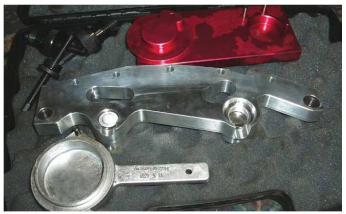
When installing the variable valve timing actuators on Double VANOS, you'll need these special tools to properly set the gear depth position. These are available through your local BMW dealer's parts department.
