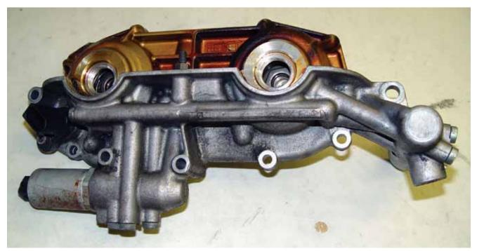
Double VANOS was the next evolutionary stage of BMW variable valve timing. This system advances the intake cam and retards the exhaust cam through a range of up to 40 crankshaft degrees for the former, and 25 degrees for the latter. It adds complexity, but enhances power output and efficiency.
