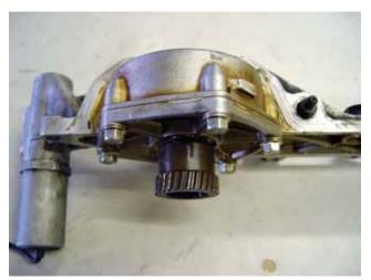
When installing the single VANOS unit, you have to make sure the gear is in its retracted position. In other words, when the gear is pushed all the way in toward the VANOS unit.
