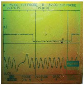
Using a dual trace oscilloscope you can monitor the crankshaft (lower trace) and camshaft (upper trace) position signals relative to one another. This is the intake cam/crank relationship on a 2000 M3. After activating the solenoid, you should see their relative positions change.
