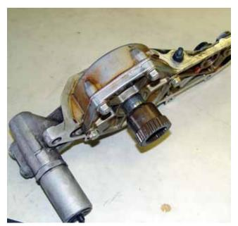
The first VANOS unit, which debuted in '92, has one helical-gear mechanism for advancing the intake cam. It only featured two phase changes, but allowed for a combination of smooth idle and improved mid-range and top-end power.
