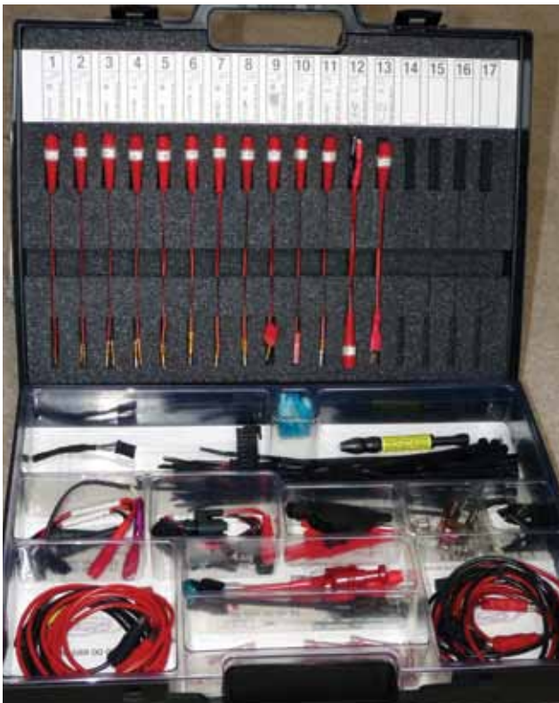
This Mercedes-Benz Electrical Test Kit Adapter Set is essential in not only ensuring good contact, but it also avoids the damage to the factory harness that might be caused by jamming an unsuitable object into the connectors when testing.
