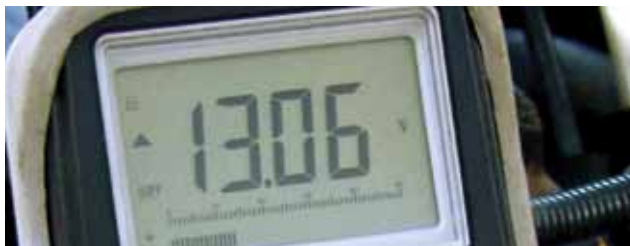
Except on the latest models with the "energy management" charging system, if you're seeing a reading this low across the battery with the engine running, you've found trouble.
