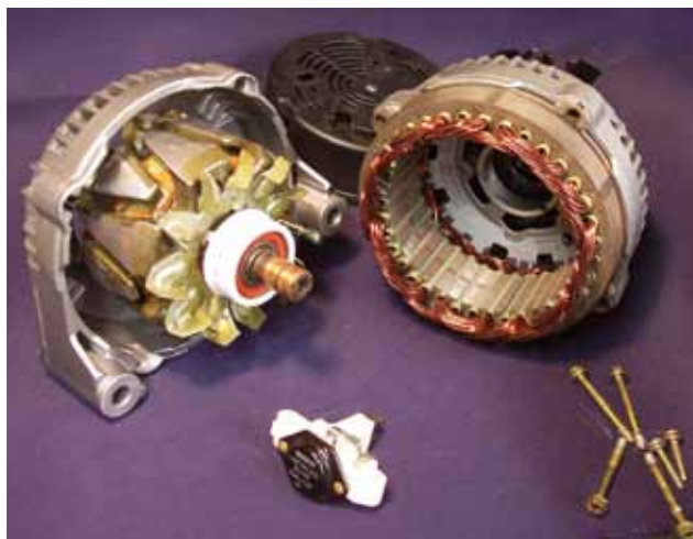
A modern AC generator/alternator should last a long, long time, but typical failures are blown diodes and worn-out brushes.
