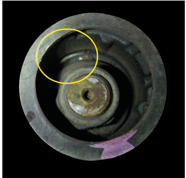
A careful visual examination will tell you a lot, such as how excessive motion has worn a "clean" spot on this strut top, which can be identified from under the hood.
