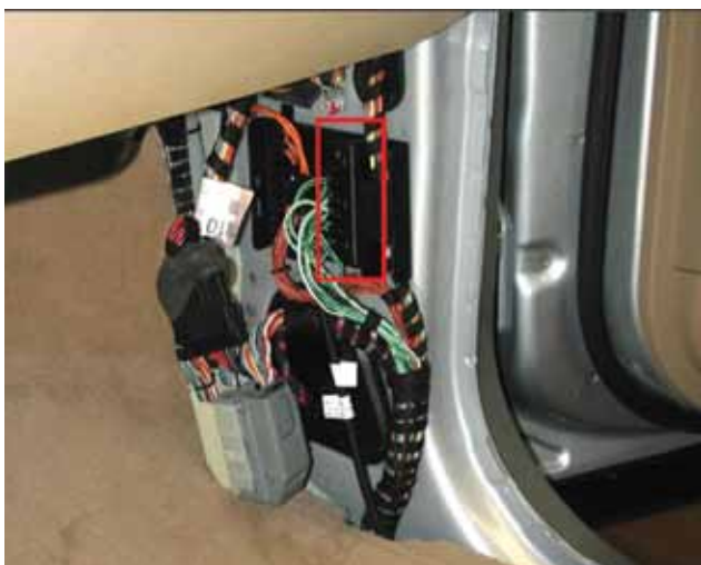
Engine CAN connector location (courtesy MBUSA).
