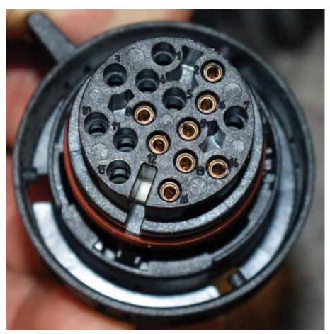
The Mechatronic control unit plug does not need many pins since most of the wiring is internal. Here we have the power supply, ground, and CAN data lines. Make sure the plug is not leaking. If it is, you can replace it.
