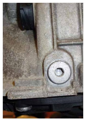
This is the fill plug on the Mechatronic transmission. Keep in mind the transmission needs to be in a specific temperature range before you can remove the plug and see if the level is correct. Run the transmission through all gears before you check the fluid level. You will also need to fill the transmission at this hole. It will be near an exhaust pipe, so protect yourself from the heat.
