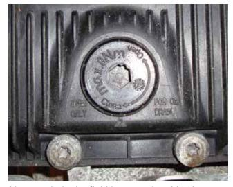
You can drain the fluid by removing this plug. Don't over-tighten past the marks on the plug as you can crack the housing and cause a leak. If you are changing the fluid, save and measure it so you know how much to put back in. BMW recommends only its own transmission fluid for these units.
