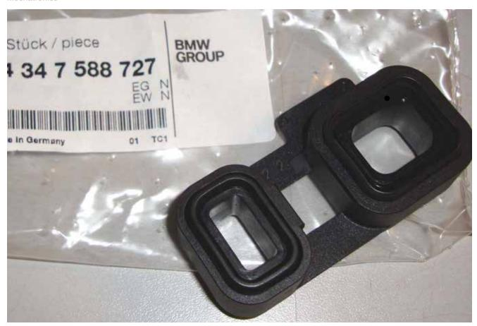
Here is the seal that contains the pressure between the Mechatronic control unit and the transmission pump. If this seal leaks the transmission may have problems moving into and out of gear. It is one of the few serviceable items inside the transmission, so it is a good thing to replace if you need to pull the valve body down.
