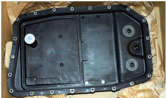
The plastic transmission oil pan should be one of the tips that let you know you are working on a Mechatronic transmission. Do not remove the pan when the transmission is hot as it can become distorted as it cools. Also, use a torque wrench when reinstalling to prevent over-tightening and cracking.
