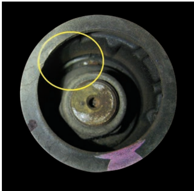
A careful visual examination will tell you a lot, such as how excessive motion has worn a "clean" spot on this strut top, which can be identified from under the hood.
