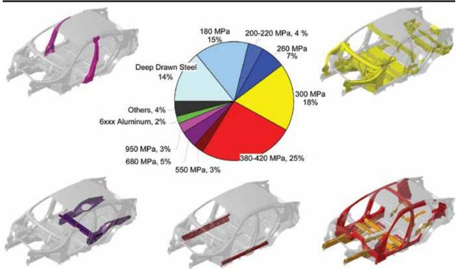
BMW "Body in White" color-coded schematics delineate the mix and location of AHSS, UHHS, aluminum, and other materials that comprise its models. For the BMW X6 shown above, BMW calls for several different joining technologies — MIG welding and brazing, spot welding, bonding, riveting and others — depending on the part being repaired. Consult ISTA for details.
