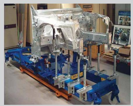
The 2004 BMW 5-Series is built with both aluminum and a variety of steels. The front end from the firewall forward is aluminum with the passenger compartment and rear section constructed from various steels. From an equipment viewpoint, BMWNA currently has approved the use of a Car-O-Liner bench fitted with a Car-O-Flex fixturing system and a Car-O-Tronic measuring system. However, the repair procedures required for aluminum parts are much different from those of the steel parts.
