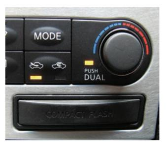
Vehicles equipped with the HDD will have a compact flash port somewhere on the dash that looks like this. It cannot be opened with the vehicle on.
