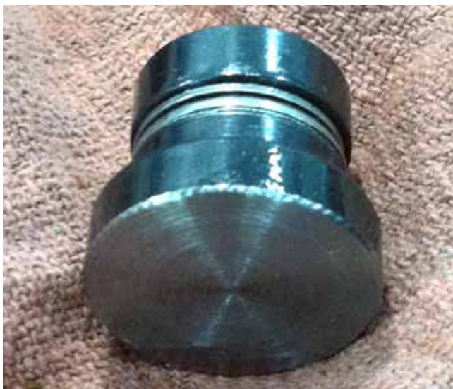
If you use a roller cam you have to use something to keep the cam from walking in and out of the block. Just make sure you've got end play on the cam after installation.
