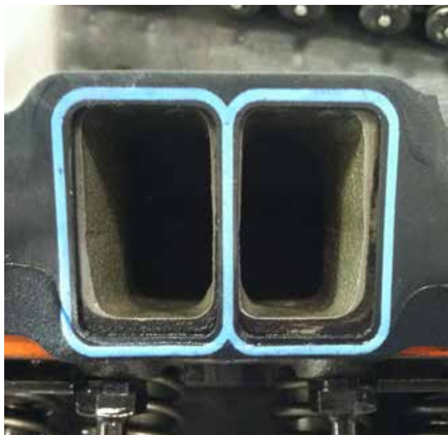
You can see the impression where the intake sealed on the gasket. Not much to hold on to!
