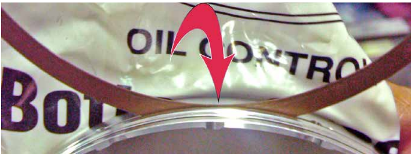
Look closely -- you can see the ring stands proud of the groove. Minimum safe back clearance is 0.005 in.
