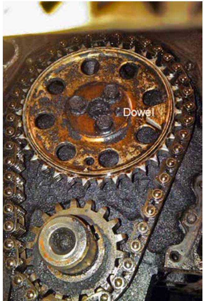
Old school: On traditional engines such as this 1967 Chevy 327, cam timing was determined once and for all by the position of the sprocket dowel.
