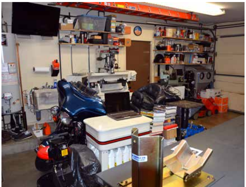
There is a large upright air compressor, a flow bench, a cold tank, a valve grinder, a lift, a seat and head machine, a blast cabinet, a water cooled TIG welder, a custom work stand and dozens of tools, jigs and fixtures stuffed into every nook and cranny. No excuses! You can do it!
