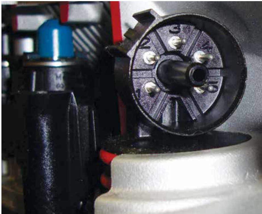
With the ETC unit moved inside the transmission, wiring to and from the control unit has been reduced. This connector is for the later 724.2 and 725 transmissions. Pins #1 and #2 are the CAN C lines and voltage is supplied on pin #5. Pin #3 is the wake-up signal from the EIS and lets the ETC unit know the key has been turned on or off.
