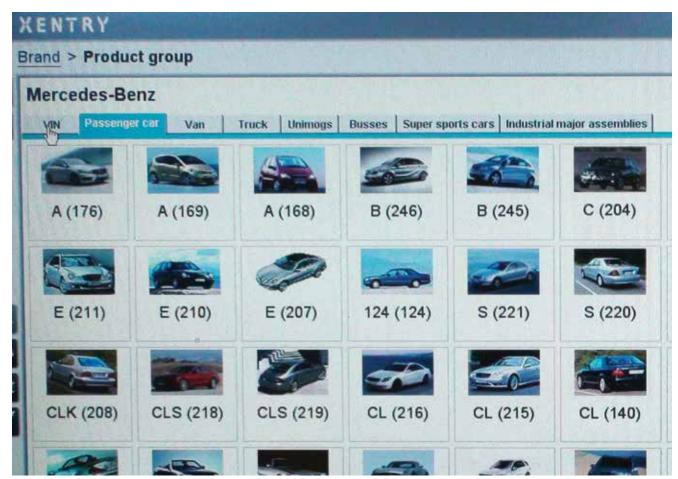
You can select the vehicle yourself if you are familiar with the Baumuster number, or you can select the VIN tab to enter the specific VIN. The SDS control unit will automatically query the vehicle for the control unit installed.
