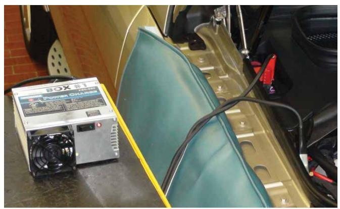
Mercedes-Benz vehicles are electronics-intensive. With the ignition key on for long periods of time, you can discharge the battery. It is always a good idea to have a battery maintainer (commercially available) attached to the lugs on the vehicle. This is particularly important if you are going to code, flash, or program a new control unit since stable voltage needs to be supplied.
