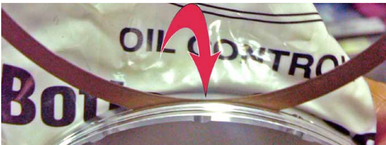
Look closely -- you can see the ring stands proud of the groove. Minimum safe back clearance is .005 in.
