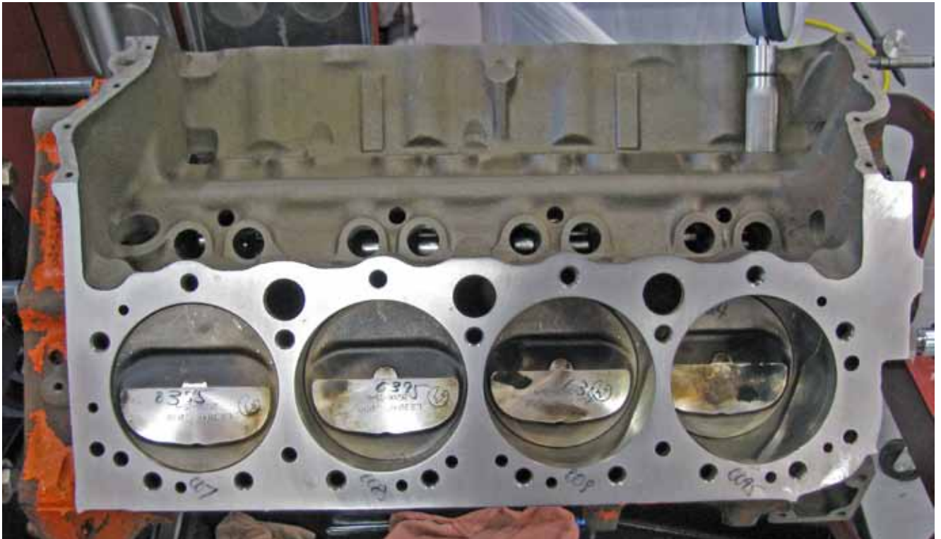
The numbers written on the pistons are how far down the bore the pistons were before we machined the deck. The numbers on the deck indicate where we ended up after machining... quite a difference! (Top: Driver's side; Bottom: Passenger's side.)
