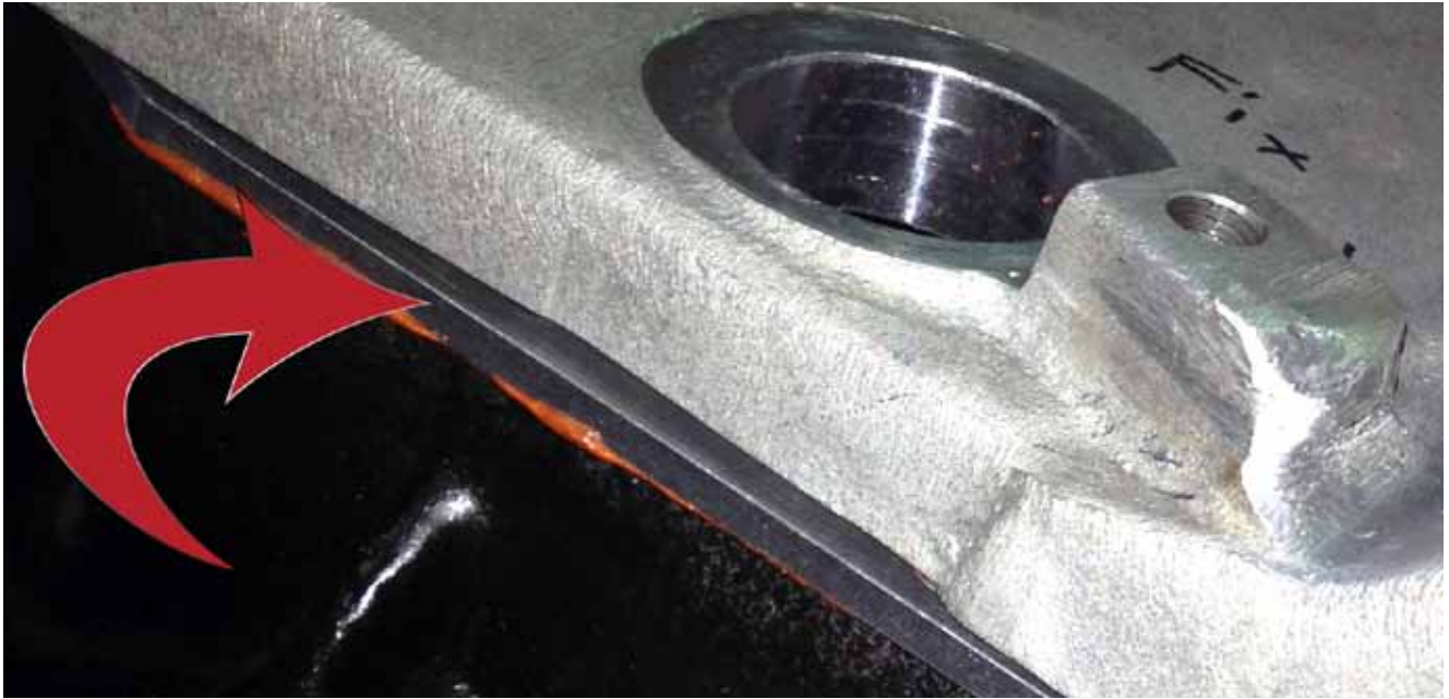
As you can see, a thin aluminum filler block is used to take up excess space between the china rail and the intake manifold. You can fill this gap with RTV, but why take the chance?
