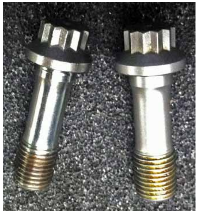
Rod bolts run $15 to over $50 each, but even at that they are cheap insurance. Never chase the stretch or you'll have to replace them all.
