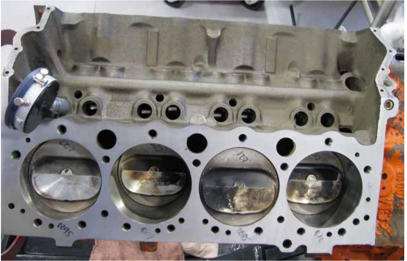
The numbers written on the pistons are how far down the bore the pistons were before we machined the deck. The numbers on the deck indicate where we ended up after machining... quite a difference! (Top: Driver's side; Bottom: Passenger's side.)
