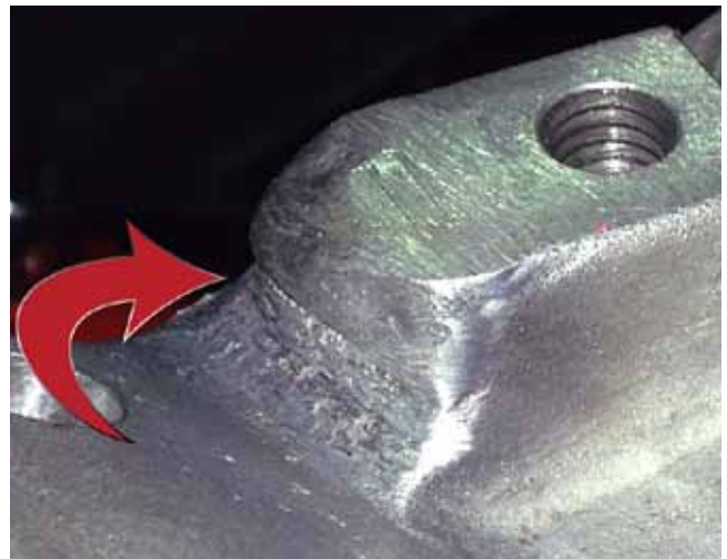
I added on about a half of an inch to the mounting boss so the distributor could be properly tightened.
