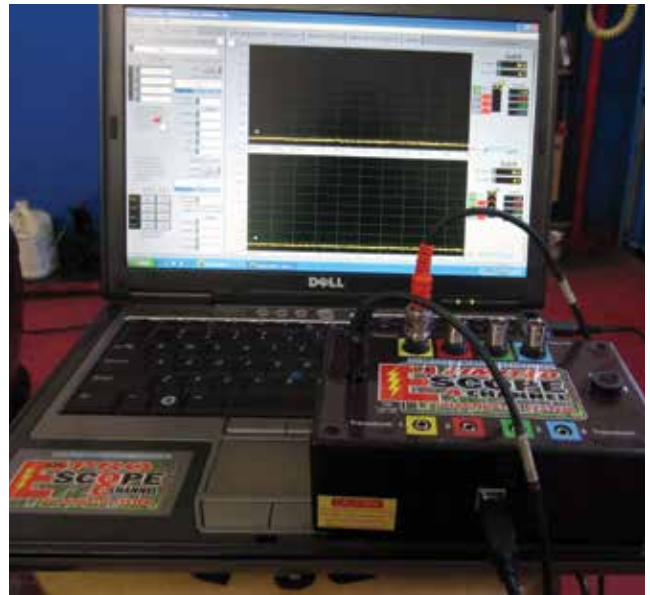
Here, a lab scope and an amp clamp are connected to a 2005 BMW 330i to test how long it takes the modules to power down. Lab scopes offer us the opportunity to “set it and forget it.” We can see at what time intervals modules go to sleep by putting the lab scope into deep record.
