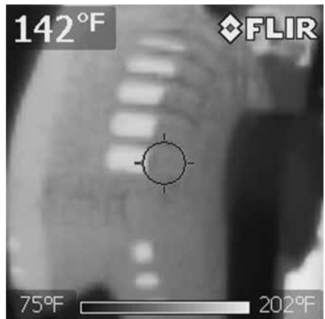
Here, a FLIR black-and-white thermal imager nails a bad alternator. It is "glowing" because an amperage draw is making it hotter than the rest of the engine compartment KOEO.
