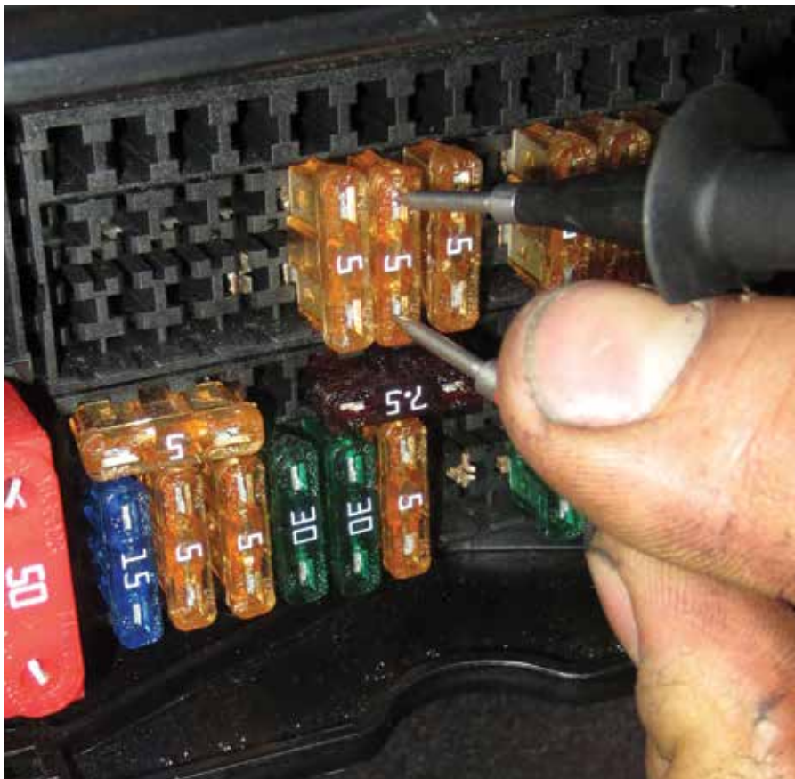
Measuring V-drop across fuses is quick and easy.
