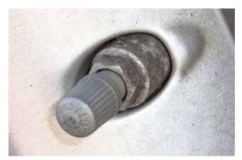
When trying to determine if you're working with an indirect or direct system, look for the lock nut holding the sensor to the rim. This means it is a direct system. Use only plastic valve caps because galvanic action will corrode the metal type on the valve stem making them difficult to remove.
