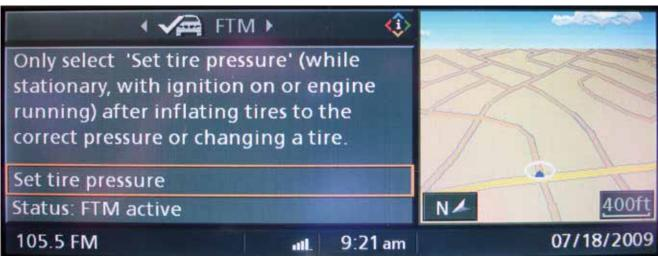
If the vehicle has a NAV screen, use the soft-key reset with the iDrive. After pushing the iDrive button, scroll left or right to the FTM screen, then select "Set Tire Pressure." After answering "Yes," the status bar should read "initializing." Now, drive the vehicle until the individual wheel pressures are displayed in the NAV pictogram.
