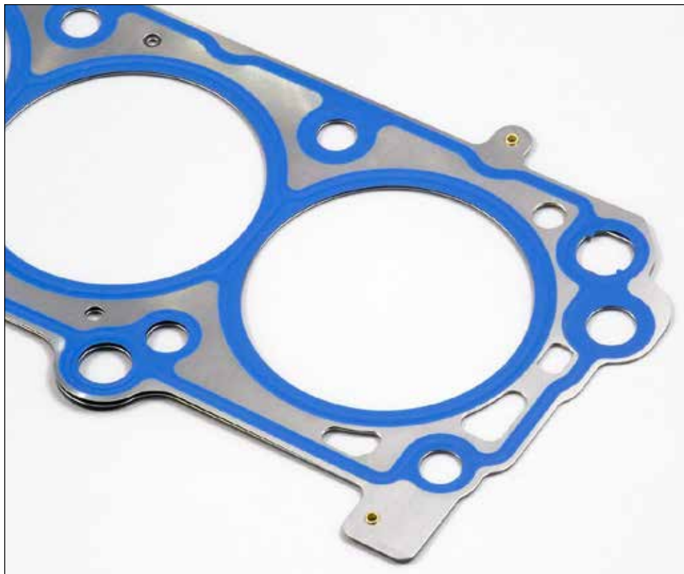
The Ford 4.6L "modular" V8 was the first domestic engine to use an MLS head gasket. This modern version for that application has selective silk screened polymer over critical sealing areas.
