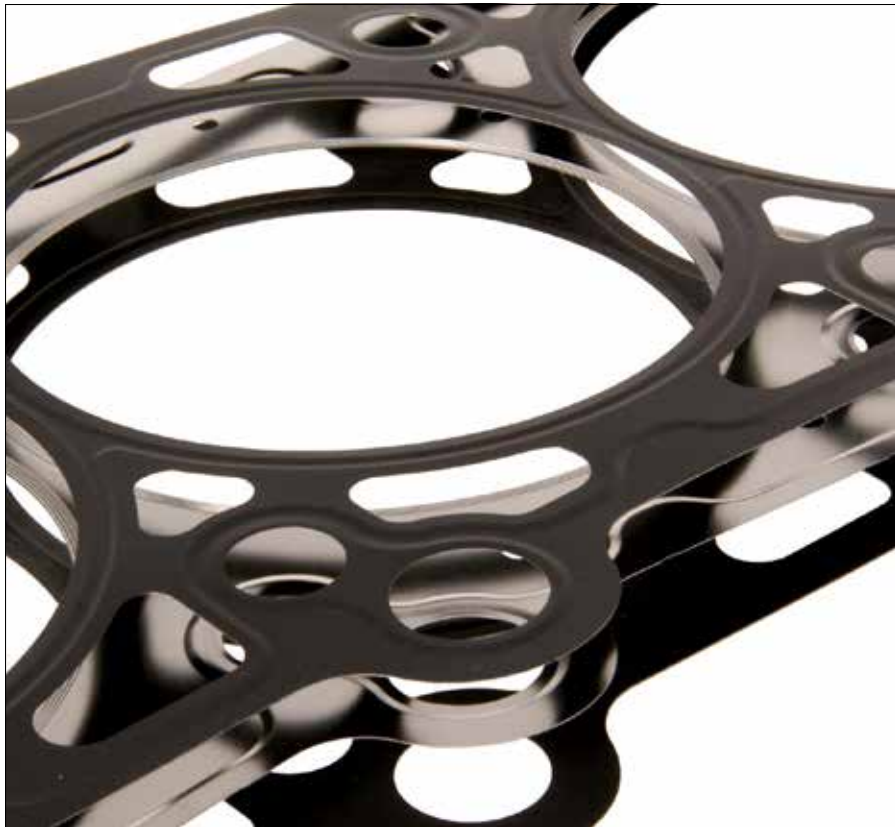
The top and bottom layers are hardened stainless steel and have raised beads called embossings on their surface, which increase clamping force where needed.
