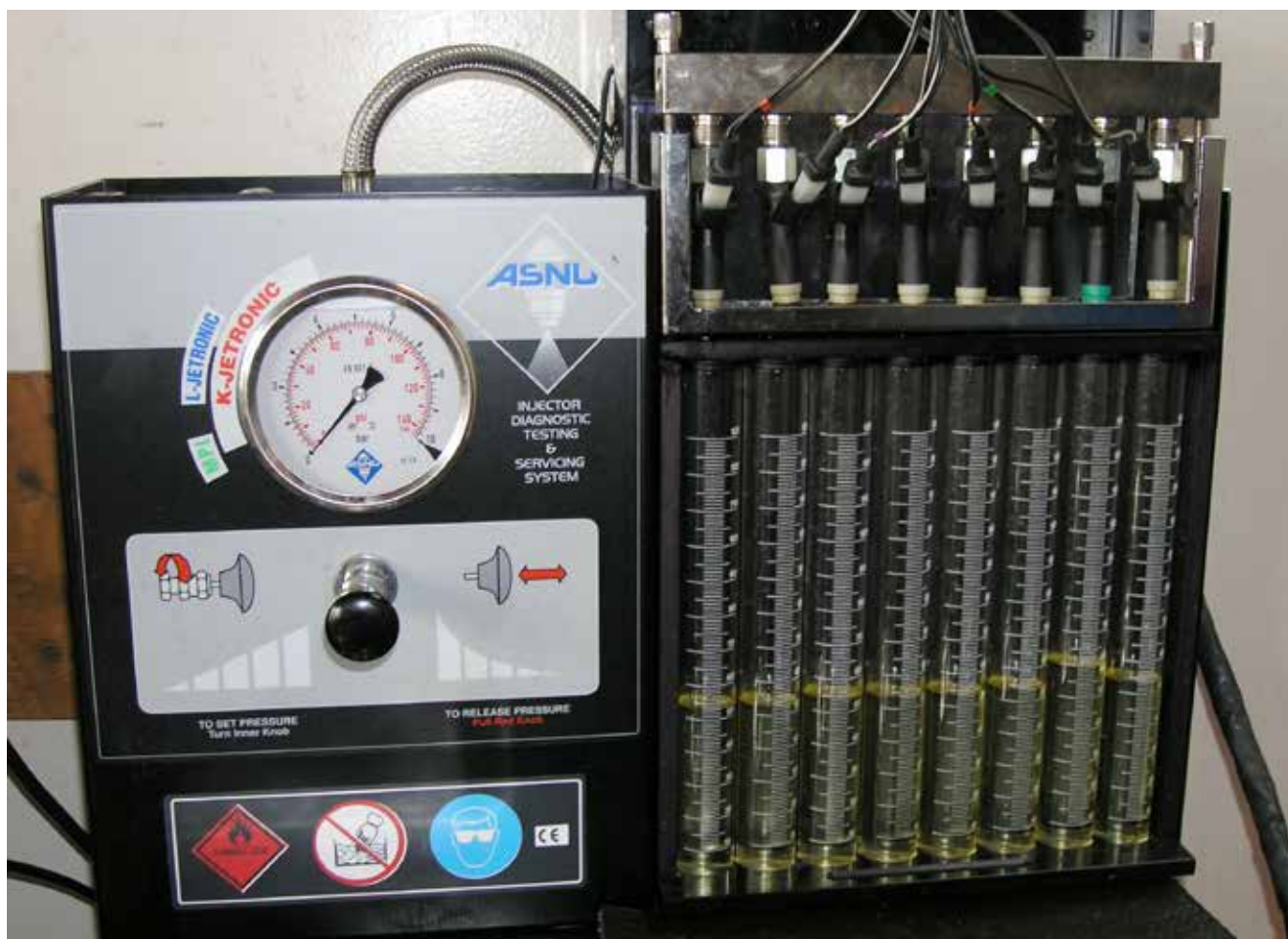
A fuel injector bench is the best way to be sure your injectors are flowing properly.
