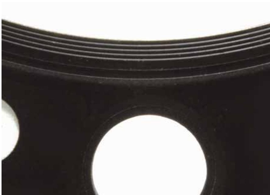
In this close-up, you can see the concentric "Wavestopper" rings around the cylinder. Each ring is capable of acting independently of the others to maintain load on the gasket even during the hardware distortion caused by heavy loads.
