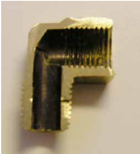
A 90-degree elbow amounts to a substantial restriction in the flow of gasoline.
