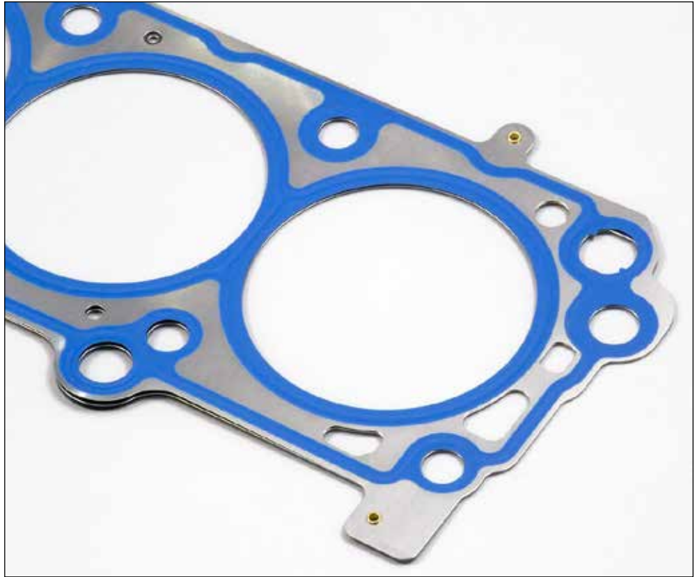
The Ford 4.6L "modular" V8 was the first domestic engine to use an MLS head gasket. This modern version for that application has selective silk screened polymer over critical sealing areas.
