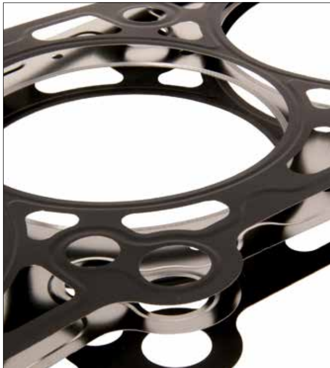
The top and bottom layers are hardened stainless steel and have raised beads called embossings on their surface, which increase clamping force where needed.
