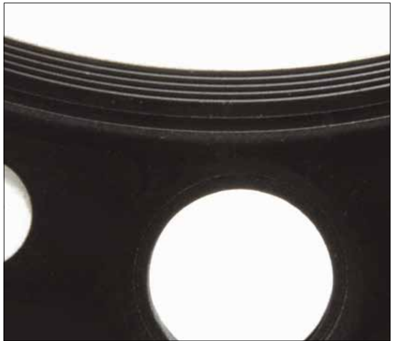
In this close-up, you can see the concentric "Wavestopper" rings around the cylinder. Each ring is capable of acting independently of the others to maintain load on the gasket even during the hardware distortion caused by heavy loads.
