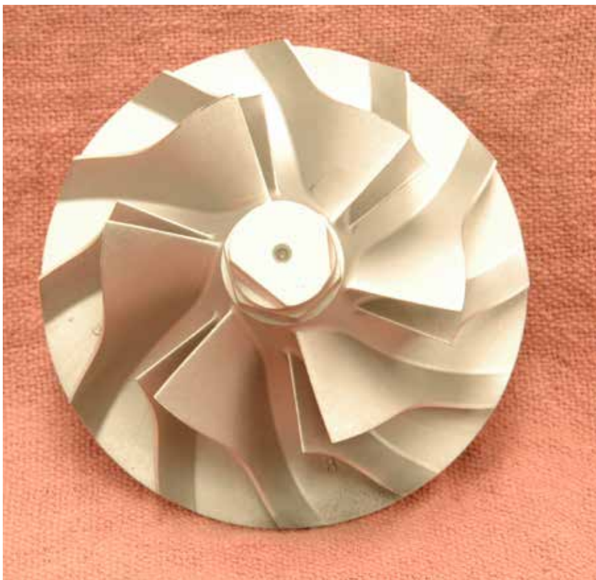
Boreless compressor wheel. Note the compound curves and flow path from inducer to exducer.
