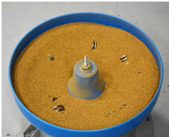
The polishing rig is a repurposed cartridge tumbler.
