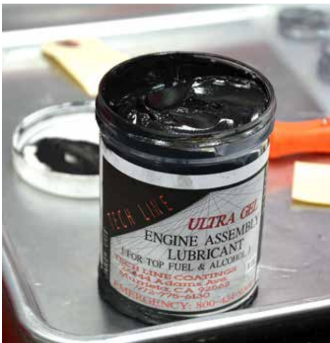
Use lube to prevent galling at retainer and spring seat.
