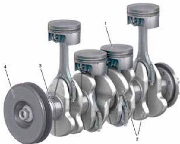
The bottom end looks indestructible. The crank, rods, and pistons are all forged.
