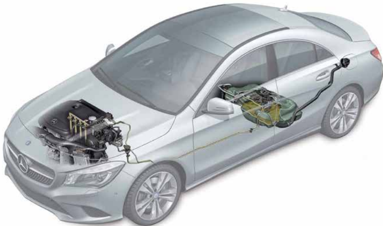
A low-pressure pump moves gasoline from the 50L high-density polyethylene tank (six layers with a block layer made of ethylene vinyl alcohol to prevent hydrocarbon evaporation) to the high-pressure pump, which can generate an impressive 2,840 psi (190 bar).
