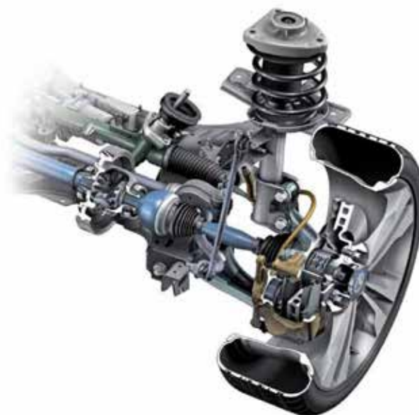
This may look like terra incognita to you -- FWD, MacPherson struts, and electrically-powered steering -- but it's thoroughly modern and works superbly. Note the long link between the stabilizer bar and the strut.
