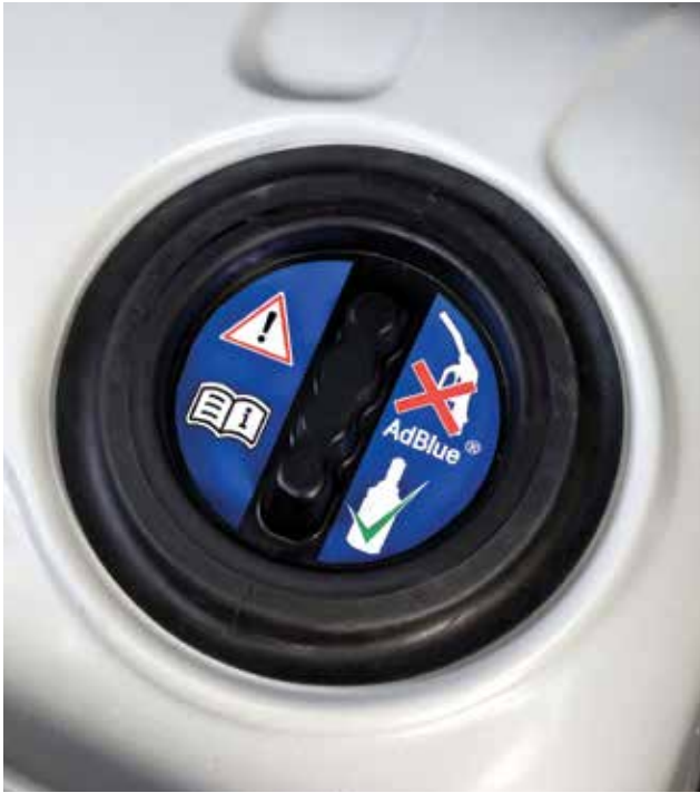
Here's what the AdBlue® DEF tank filler cap looks like. The fluid level is continuously monitored to make sure there is enough. When it gets low, a message will appear in the instrument cluster, then there will be a warning gong.
