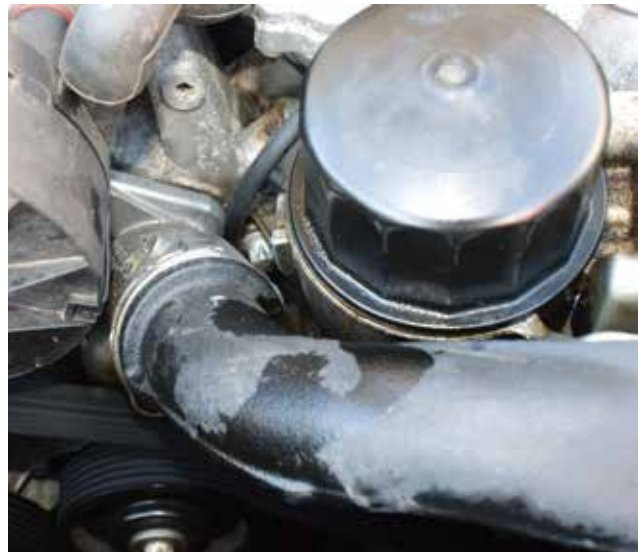
This is the e-thermostat location on a 221 chassis with the V12 engine. It is buried under the Secondary Air Pump motor and behind an idler pulley for the drive belt. WIS can help you with both testing and service procedures.
