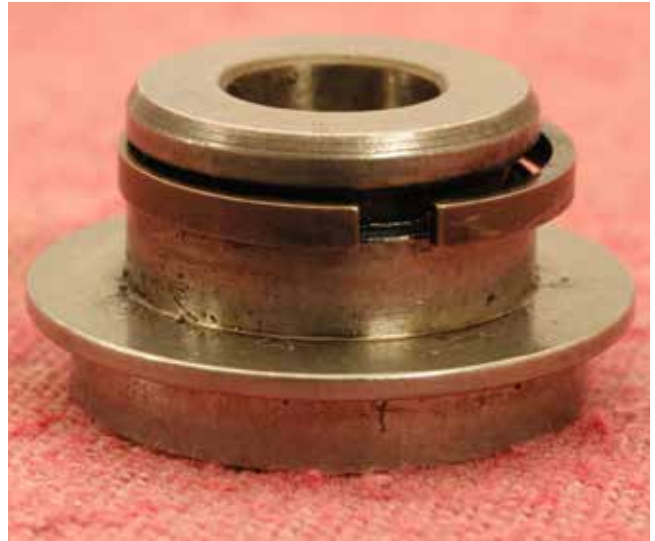
The gas/oil seal is a simple metal part resembling a piston ring.
