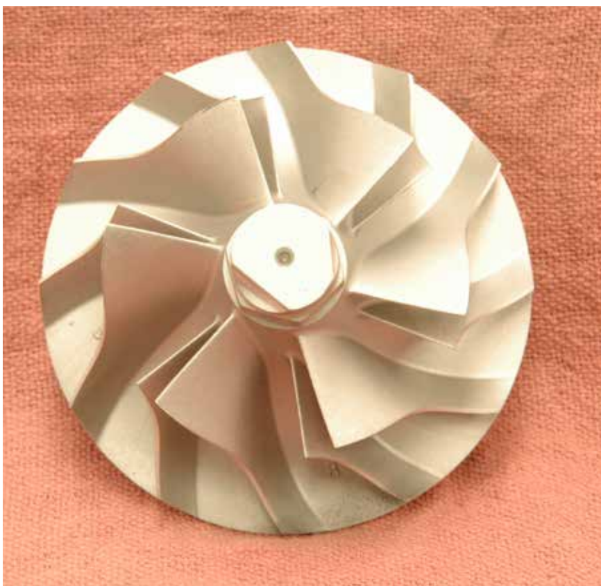
Boreless compressor wheel. Note the compound curves and flow path from inducer to exducer.
