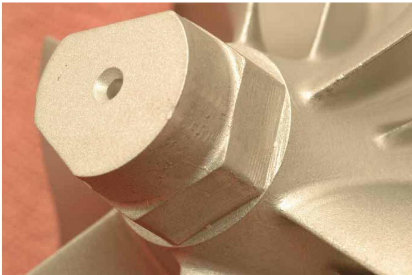
New compressor and turbine wheels are not through-bored. On this “boreless” wheel, a partial bore-through is threaded, and the wheel threads directly onto the shaft.
