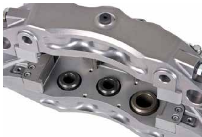
The differential bore sizes are clearly visible in this six-piston caliper. Engineers juggle this to even out the force on the pads (courtesy StopTech).
