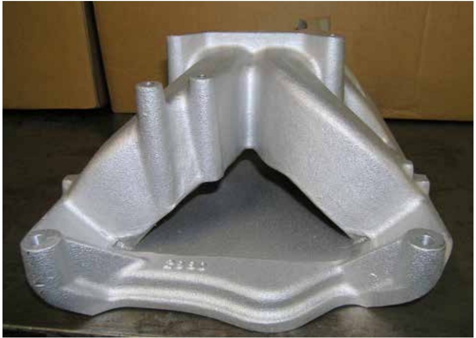
This Edelbrock Air-Gap intake manifold will help the engine make maximum power at high rpm operating conditions.
