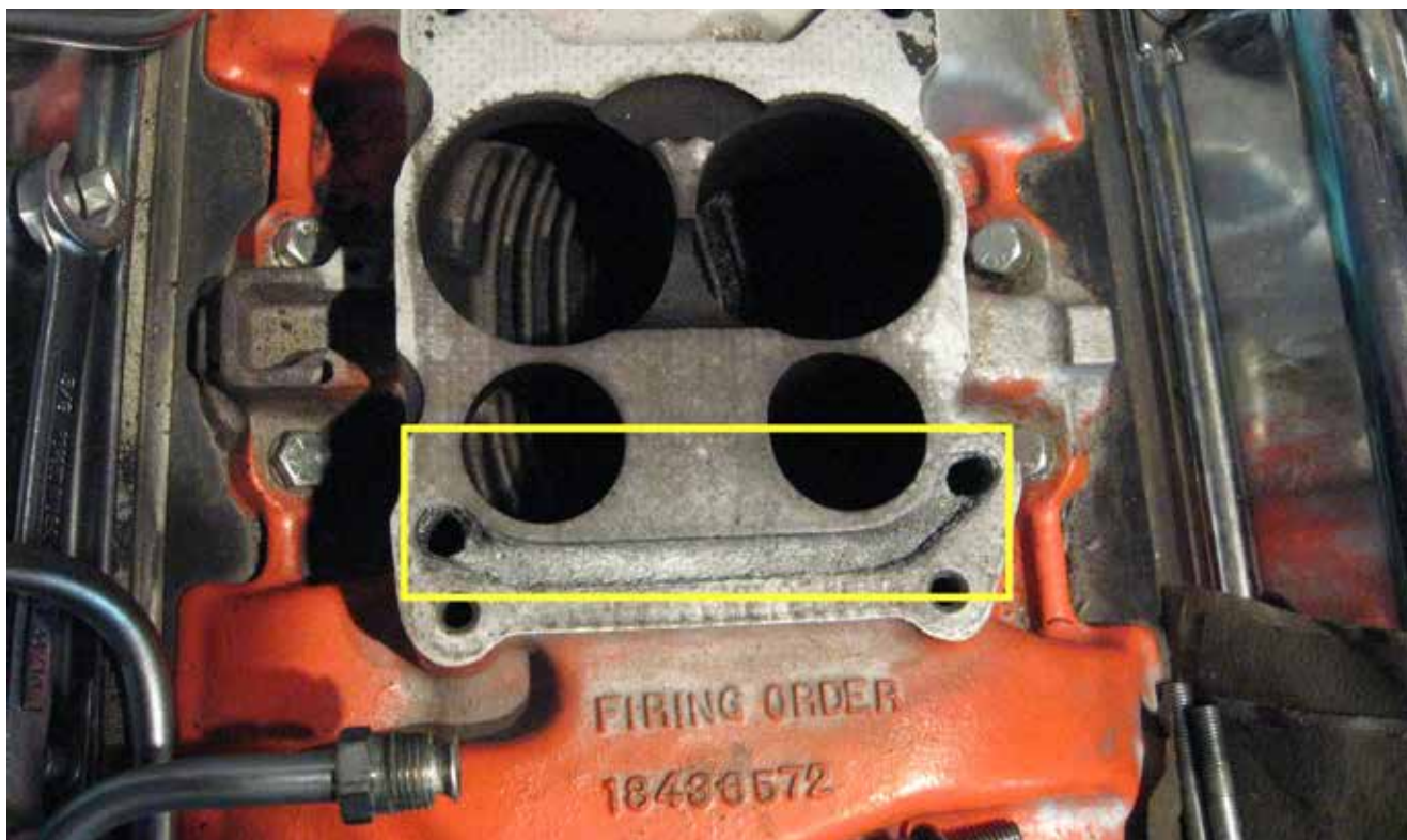
General Motors used exhaust gases to aid in fuel vaporization, but this tended to overheat the carburetor and led to vapor lock problems.
