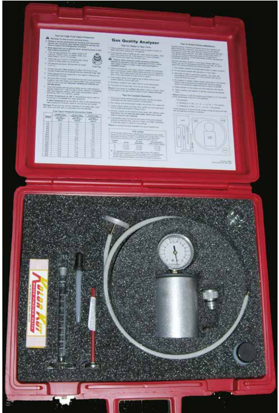
This gasoline quality analyzer from OTC/SPX can be used to check how volatile the gasoline is.
