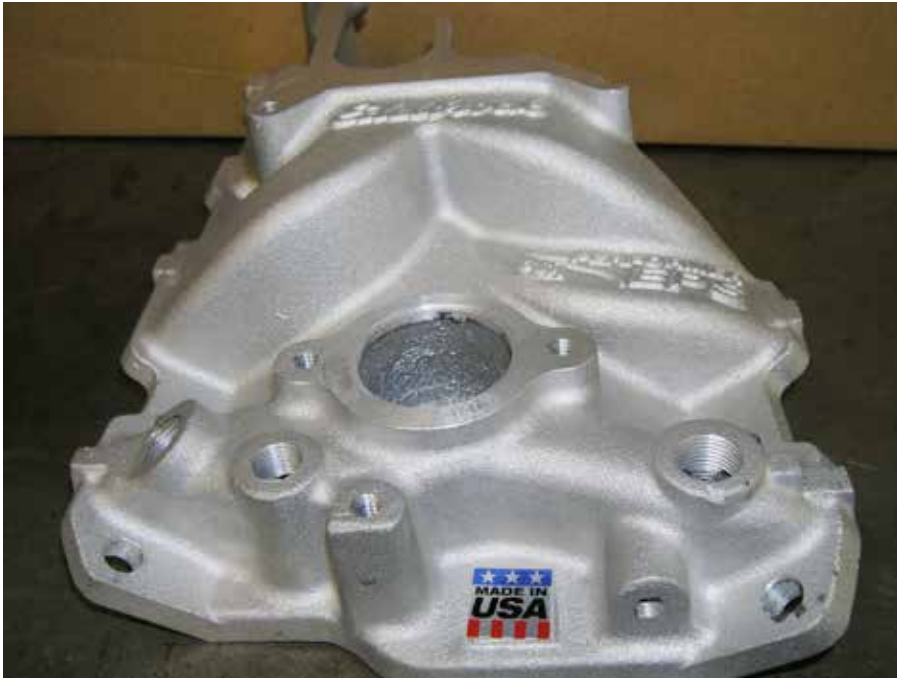
A dual-plane manifold is a good choice for power over a wide range of engine rpm.
