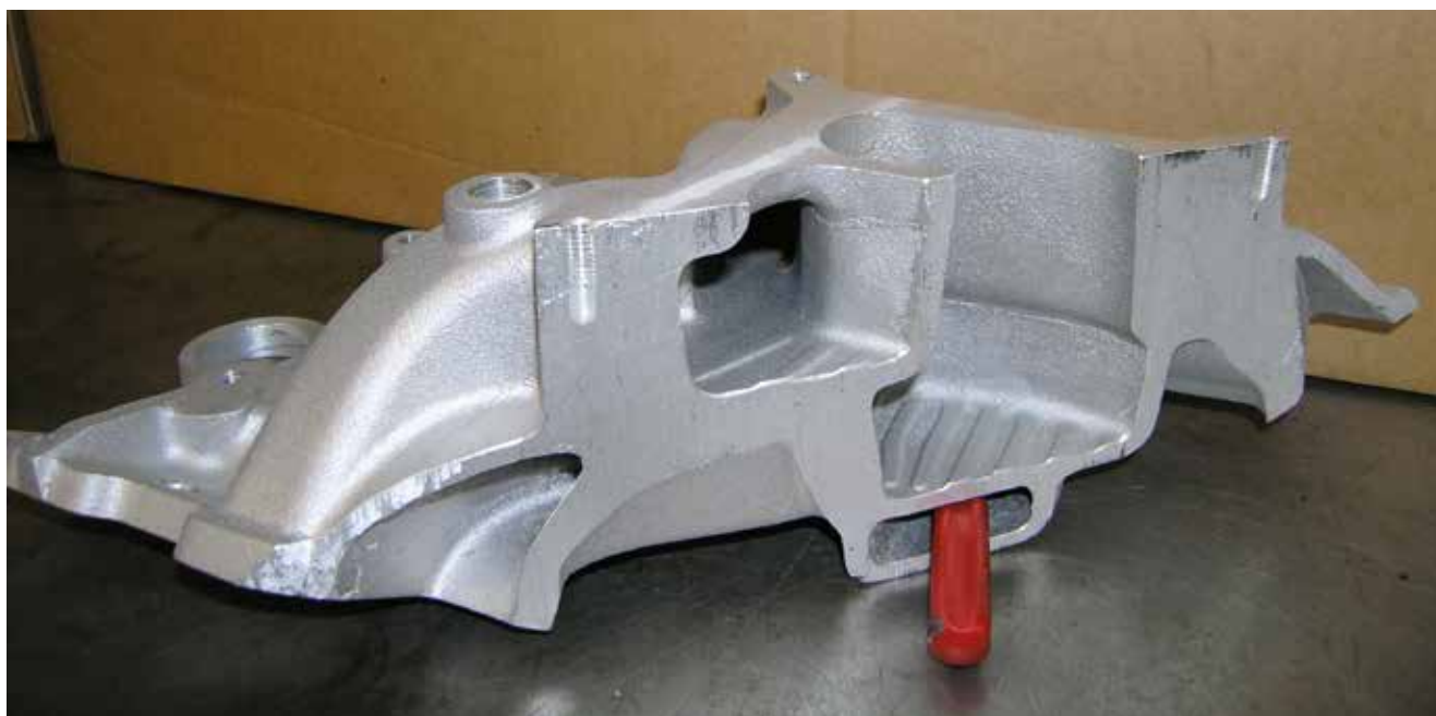
This cutaway of an Edelbrock dual-plane intake manifold shows the exhaust crossover passage that's used to aid in fuel vaporization.
