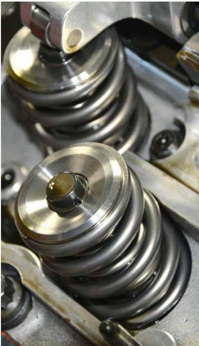
Titanium retainer and lash cap in place.
