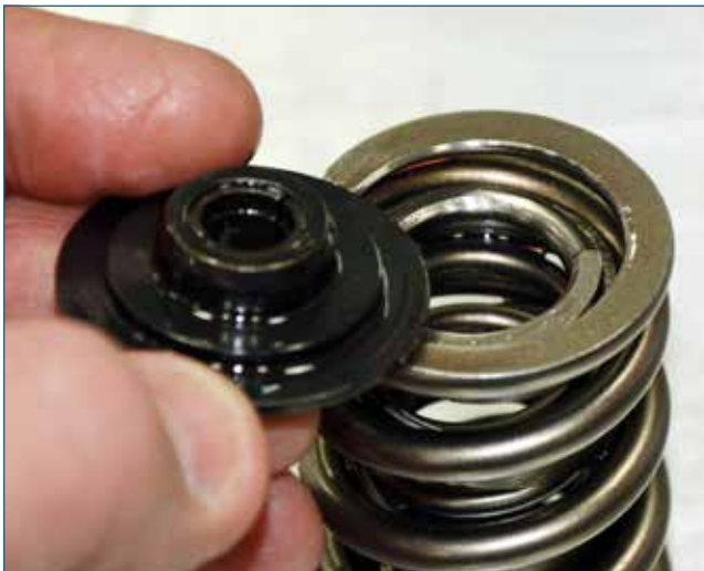
Cannot check springs without the retainer.
