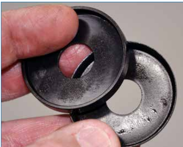
Seats are part of the installed height.
