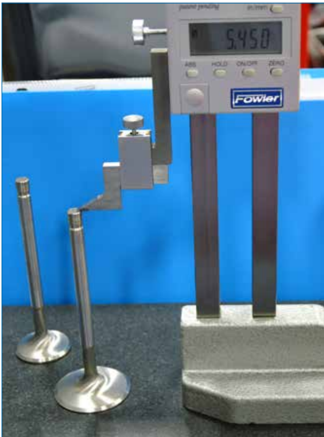
Intake valve stem height.
