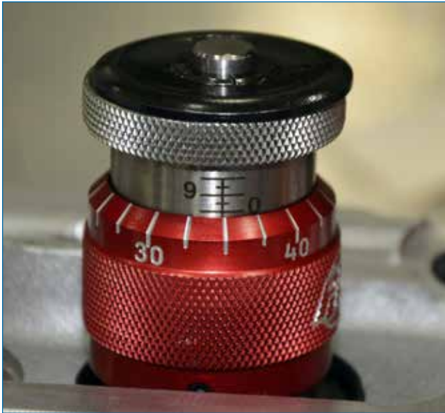
Intake installed height.
