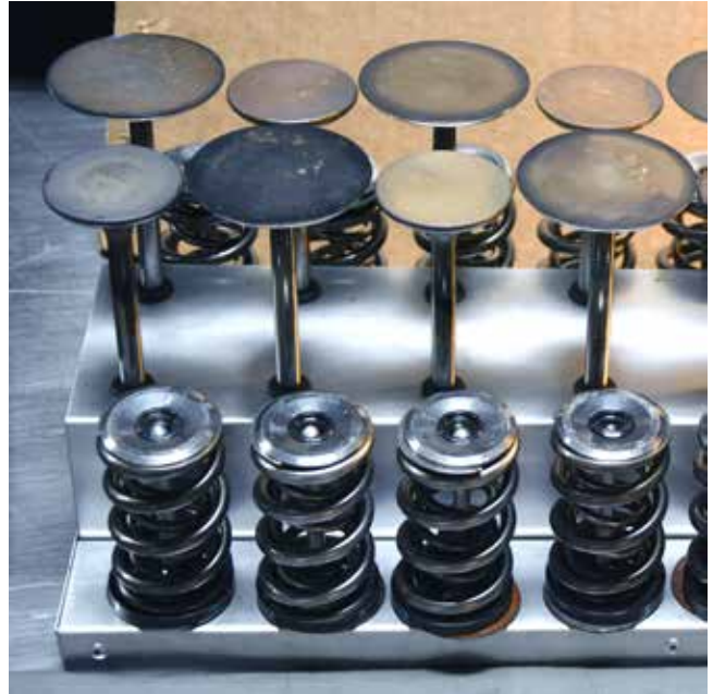
Loaded spring and valve tray.
