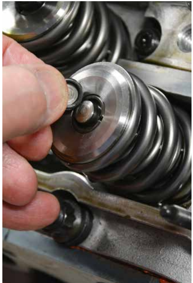
Have to use steel lash caps if there are no hardened inserts at valve tip.
