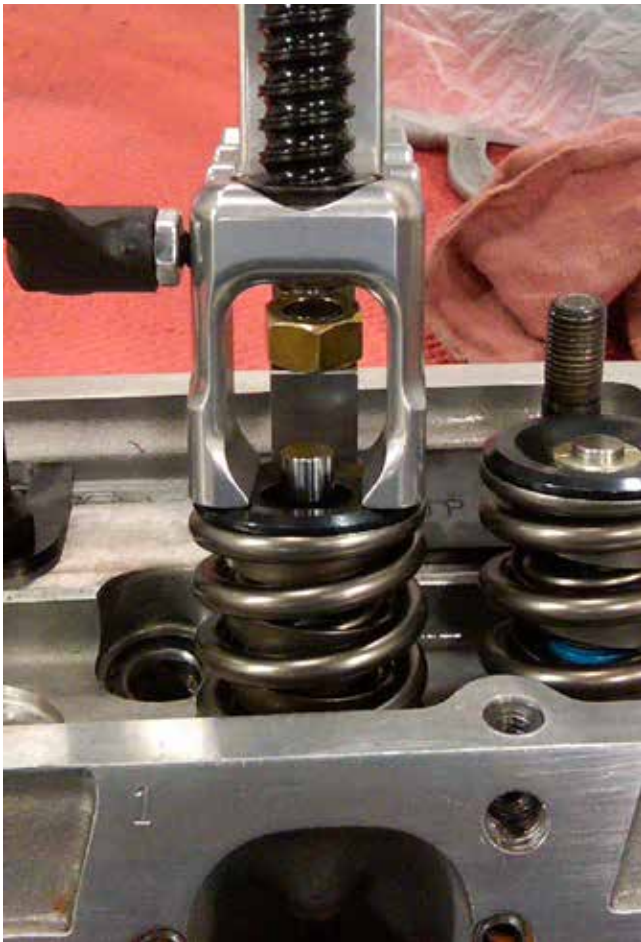
Buxton compression in operation.
