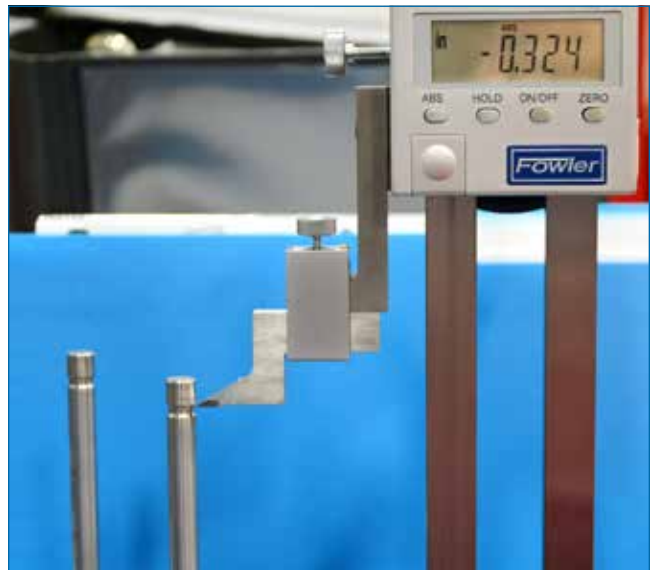
Autozero, then measure tip height.
