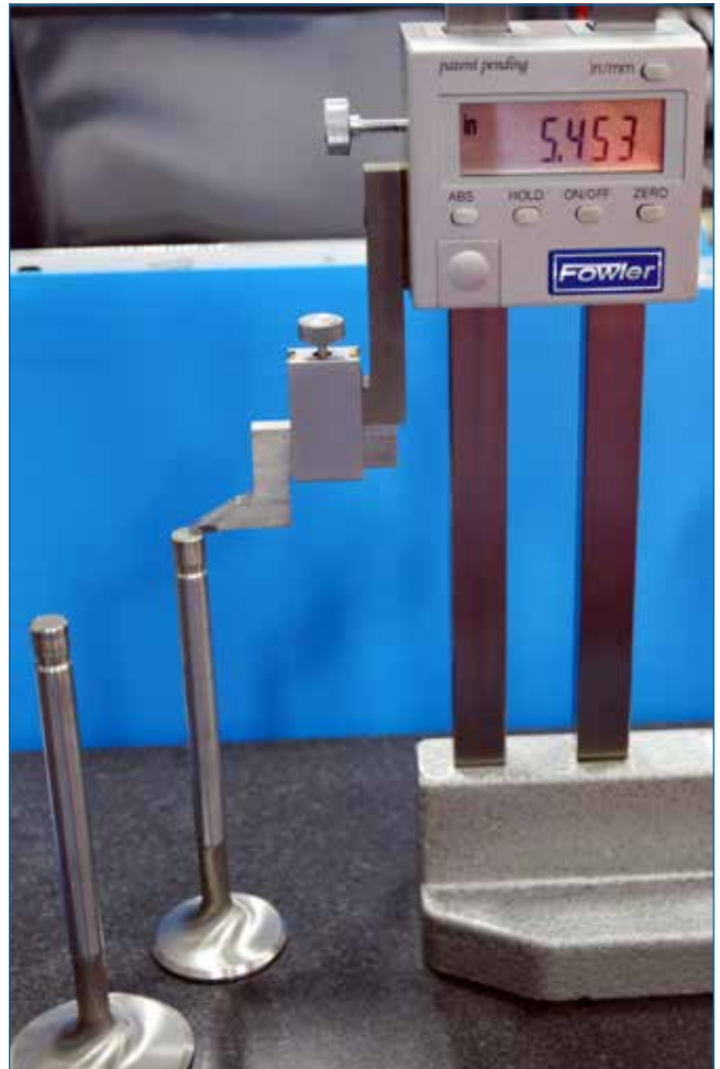
Exhaust valve stem height.
