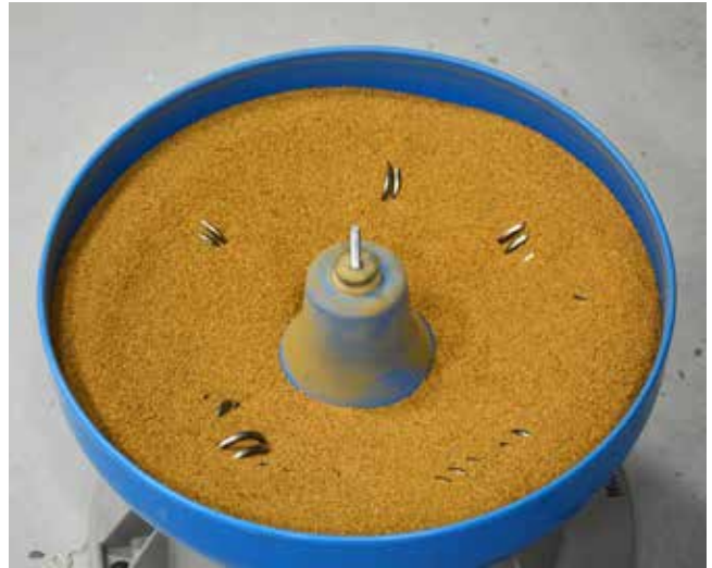
The polishing rig is a repurposed cartridge tumbler.
