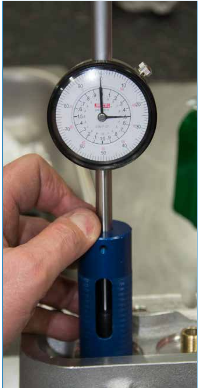
Valve seat height check.
