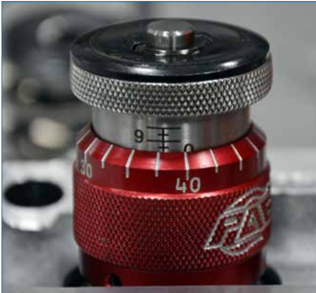
Exhaust installed height.
