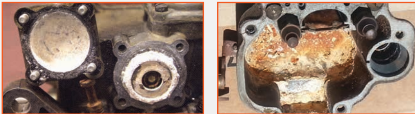
Ethanol Attacks Carburetors & Mechanical Fuel Pumps.
