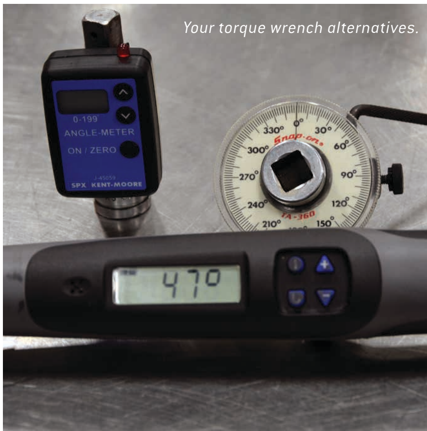
Center your hand over the notch of a digital torque wrench to assure uniformity.
