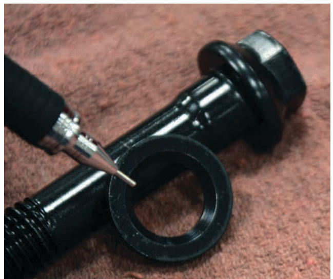
Washers must be relieved to clear the radius.
