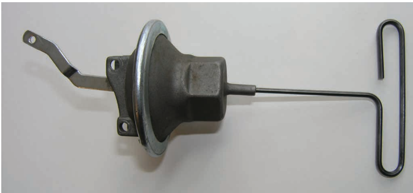
This Ford vacuum advance has an adjustable stop that is adjusted with an Allen wrench.
