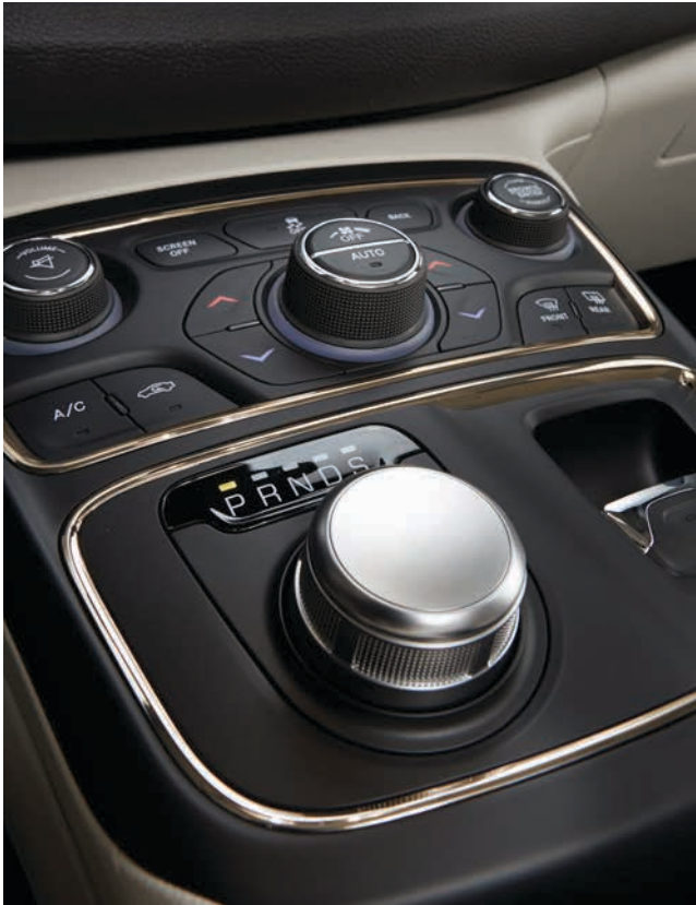
The nine-speed automatic transmission is controlled by a rotary dial.
