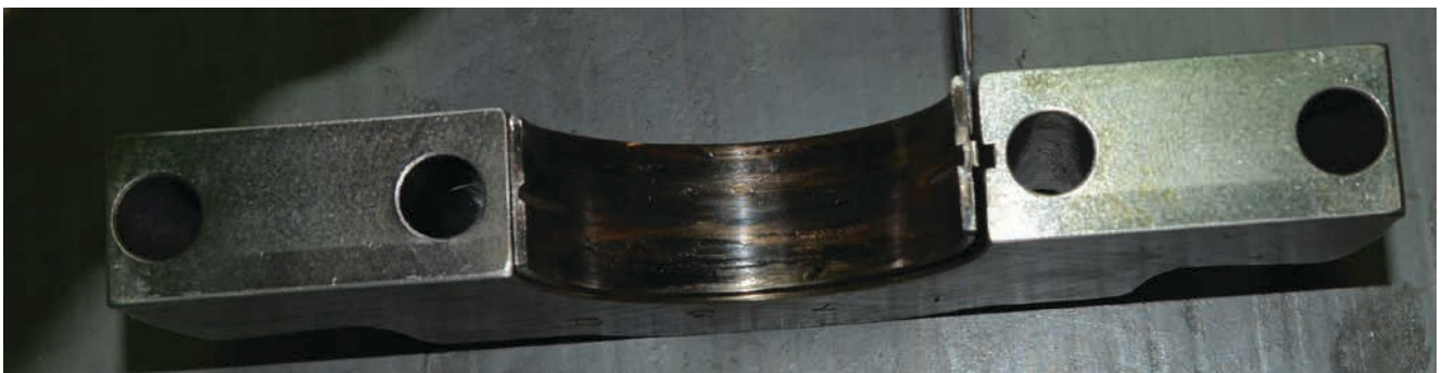
This will give you some idea of how severe a beating this bearing got before it gave up. I can stick the tip of my pocket screwdriver into the space between the main cap and the bearing.
