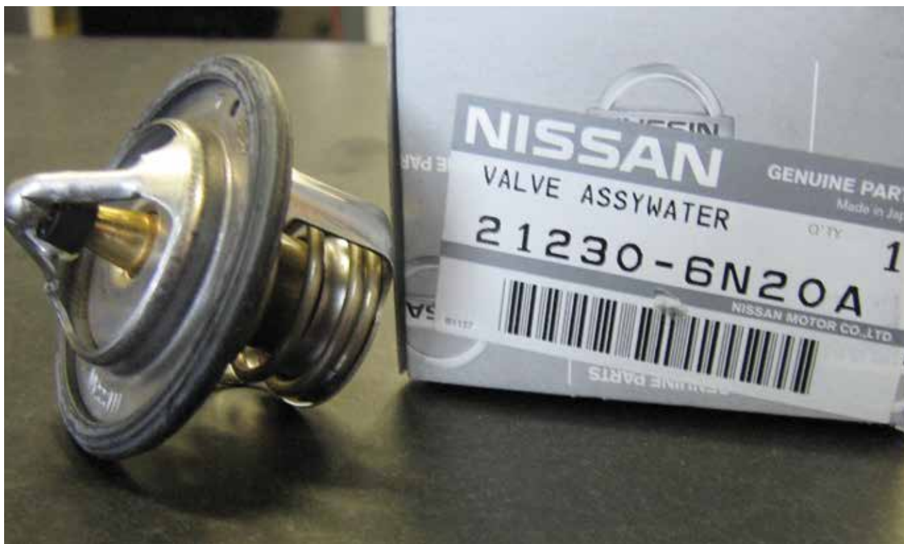
The water control valve looks similar to a thermostat in almost every respect. This one opens at a slightly lower temperature, though (171 deg. F.).
