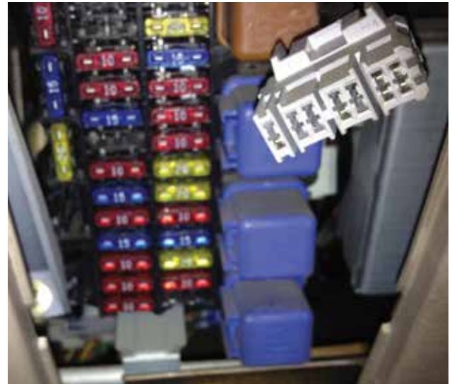
The proprietary Nissan 14-pin DLC is often found behind the fuse panel cover.
