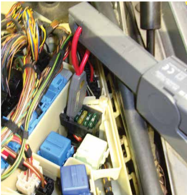
The injectors also receive a power supply feed from the fuse holder in the electronics box. By using a loop in place of the fuse, you can install a low current probe and measure the amperage draw of each cylinder.
