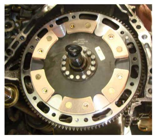
With our new flywheel, we of course installed a new pilot bearing. No sense having your input shaft wobbling around under hard acceleration stressing out the input shaft bearings. The pilot bearing is pressed into the flywheel, and make sure you have pressed it in all the way and it is fully seated up against the lip. Whether you are using a bearing driver kit or a hydraulic press make sure your tool is only applying pressure to the outside bearing race to avoid stressing the bearing.
