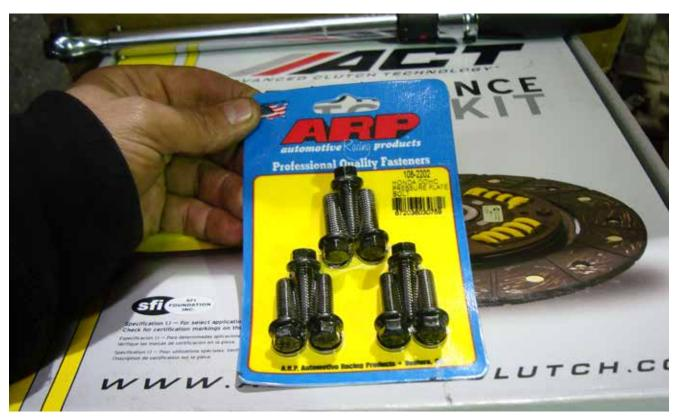
ARP makes the perfect bolt kit because most upgrades use nine bolts to secure the clutch pressure plate to the upgraded nine bolt flywheel. High-grade bolts will do a much better job of securing the clutch pressure plate under heavy acceleration.
