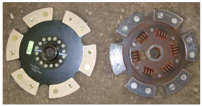
Although an upgraded six-puck clutch plate had been previously installed in the vehicle, we opted for the rigid design this time. The old clutch had springs to absorb some of the shock to the driveline when the clutch engages, which changes the weight of this part of the clutch assembly. This is more of a racing set up, and you will notice this during clutch engagement.
