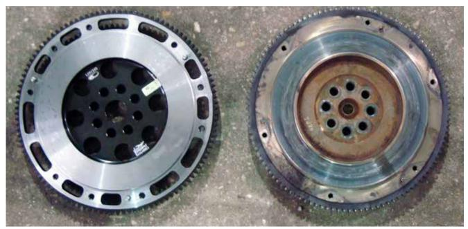
Will the huge reduction in rotating mass represented by the installation of that high-performance flywheel have negative driveability consequenses? After all, the one on the left weighs about 75% less than the stock unit on the right.
