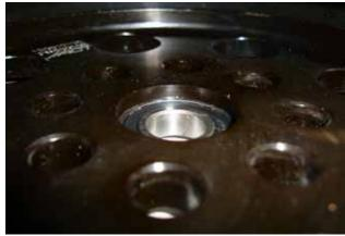
The clutch kit purchased comes with everything but the Prolite flywheel. Make sure to install or press the pilot bearing all the way in until it is fully seated up against the lip of the new flywheel.
