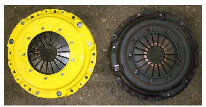
This is what makes a clutch a clutch. The spring pressure provides the clamping force to transfer the power from the crankshaft to the gearbox input shaft. We opted for the rigid disc with a torque capacity of 280 ft. lbs., this for the moment is more than the engine produces. As far as weight goes, ACT states its clutch assembly weighs about the same as the stock unit.
