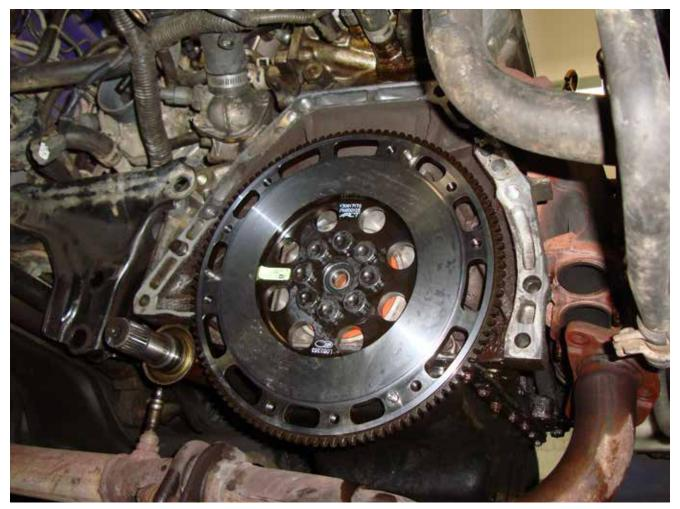
Here, new ARP bolts are being used to secure the flywheel to the crankshaft. These should be torqued down to ARP specs. The company also supplies a thread lubricant to ensure proper torque. You also might notice the new rear crank seal hiding behind the flywheel (orange).
