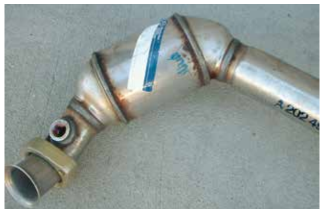
Basic aftermarket catalytic converters that barely meet EPA guidelines are notorious for having short lives. This genuine replacement unit will last as long as the original.
