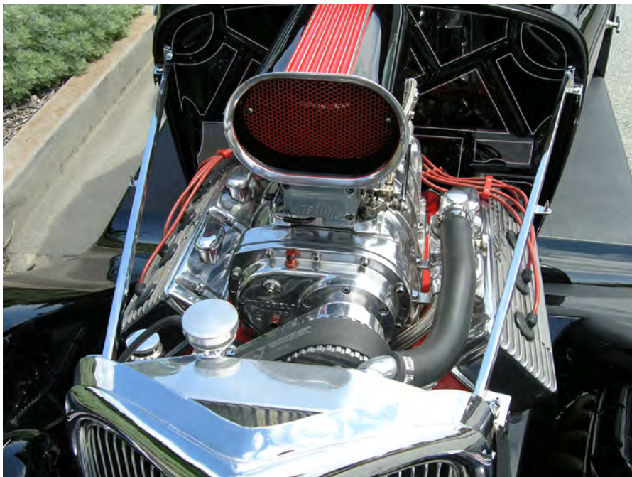
Barry Grant Road Demon Jr. blower carbs use a connection on the base plate below the fuel bowls to supply the power valves with the correct vacuum signal for the needs of a supercharged engine.
