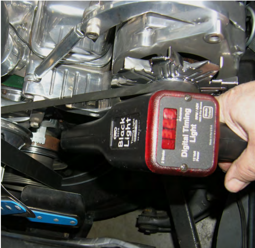
A dial-back timing light can also allow you to observe the spark advance.
