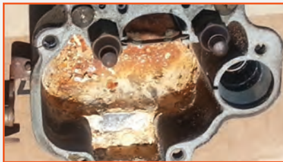
Ethanol Attacks Carburetors & Mechanical Fuel Pumps.
