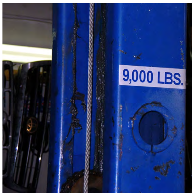
Given the increasing weight of some newer pickups, make sure the lift is rated for the heavy lifting.
