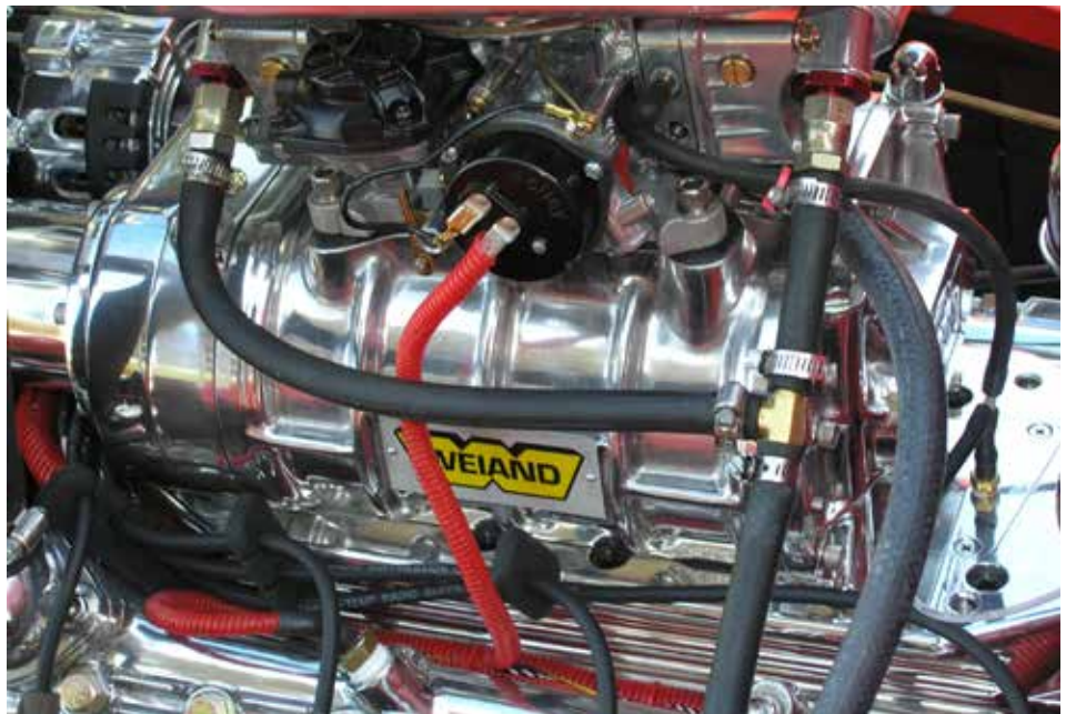
This picture shows the vacuum hose that connects to a port on the manifold below the supercharger that goes to the tube behind the choke on this Holley carburetor's boost-referenced power valve.
