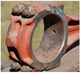
This is a racing connecting rod for a Briggs & Stratton -- Okay, I'm kidding. This is an extreme example of a connecting rod from a seven and a half by seven inch Waukesha industrial engine. I've had it for years and I pulled it out just so I could show you another world of connecting rods. It measures 18 ½ inches from center to center, uses four rod bolts and it's gun drilled to provide lubrication up to the pin bushing and the piston oil spray nozzle.
