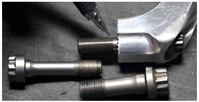
Comparing the engaged thread length on these three rod bolts reveals something that seems logical: The aluminum rod uses a longer thread engagement. While the two examples used in steel rods have nearly identical thread lengths, the aluminum rod has almost double the thread engagement. If you're threading into a softer material, you'll need more thread engagement to hold the torque without stripping. Makes sense to me.
