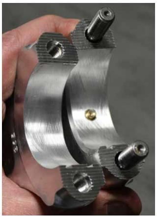
Connecting rods try to collapse inward at the parting line under tension, so keeping the parting lines solidly locked together is critical. Steel rods most often use dowels, but more interlocking surface area is engaged if you have precision machined serrations like these.
