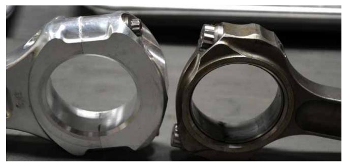
You can see how much bigger the rod big end is to accommodate the material strength and distortion characteristics of aluminum versus steel. You can also see how carefully shaped the upper shoulders of the rod are so these newer designs don't take near as much effort to install. Watch the clearance on the cam, bottom of the bores, and the block skirt areas.
