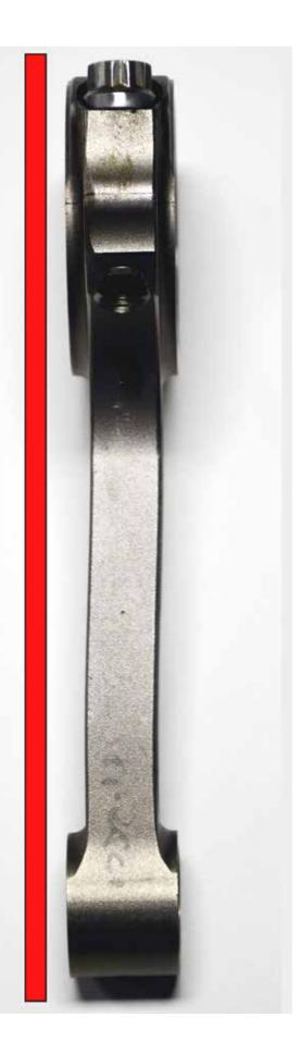
than a solid object; the cap and beam of the rod appear to be one solid piece. This is not something that can be accurately done with a torque wrench, which is more affected by thread and bolt under-head friction than by actual fastener loading. As you increase torque, this actually gets worse.
