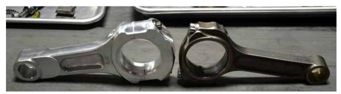
In a side-by-side comparison, the additional material used in the aluminum rod is apparent. The beam is thicker and the material around the crankpin and piston pin bores is thicker as well. Even so, it is much lighter than its steel counterpart.
