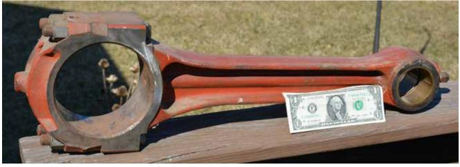
How big do connecting rods get? A LOT bigger than this one! Shipboard recip engines measure their bore and stroke in feet! This Waukesha rod measures about 18 ½ inches center to center and it's a good example of an "I" beam rod. It's a doozy... the engine it came out of was for power generation in an apartment complex and it ran at around 800 rpm.
