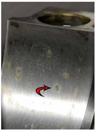
It's not uncommon to begin to see fretting and micro-welding occurring in highhorsepower applications. There are a lot of things moving and vibrating inside that engine under full load. Over three or four seasons you might notice small areas of fretting and micro-welding starting to appear. Eventually parts will have to be re-machined and bores trued.
