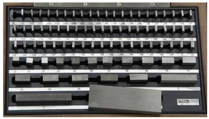
Gauge blocks like these, along with micrometer standards and pin gauges, are the only way to check your measurement equipment for accuracy. If you aren't measuring what you think you're measuring, you can't trust the results.
