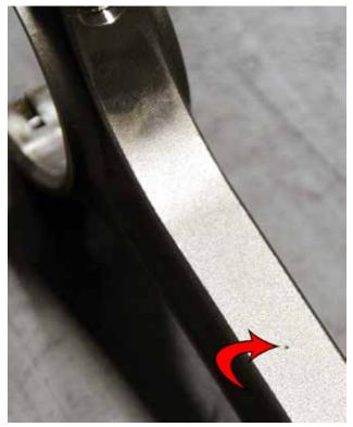
The only acceptable marks on a connecting rod beam will be the tiny dent you see here, left behind by a hardness tester used to check the Rockwell hardness of the finished product. Any mark, nick, or dent on the beam edge will certainly cause rod failure.
