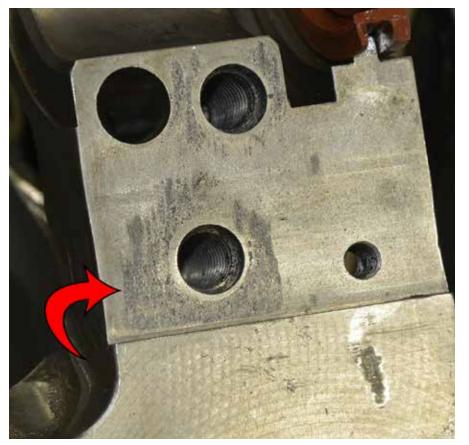
As the power levels go up, seeing this isn't completely unexpected. Even with billet caps, four-bolt mains and half-inch studs if you make enough power you're going to move things around. After three seasons this rear main cap shows what happens when you "shake things up a bit."
