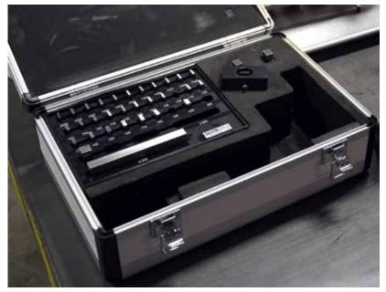
It is possible to set a dial bore gauge with a micrometer, but it is a pain and it takes time. A checking and setting fixture like this really speeds the process. The vertical fixture holds a combination of gauge blocks equal to the diameter you want to measure, and you set up your dial bore gauge by measuring between the lower and upper pad. You can also check micrometers with gauge blocks, or use them to space parts during mockup.
