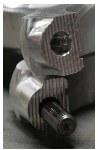
Here's a close-up of those serrations on a Bill Miller connecting rod. Very pretty work and very effective at keeping the softer aluminum rods from pulling in when the rod is under tension. If the sides pull in, they form a squeegee that wipes the oil from the journal resulting in rod bearing failure from lack of lubrication.
