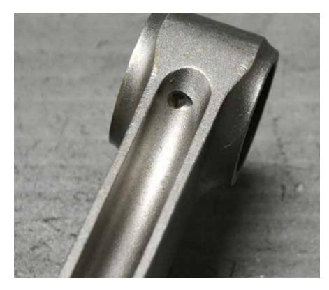
Left: Oil feed into the rod bushing may be done from above or below the pin boss. Some rods have a hole drilled on top with a chamfer to collect oil. others drill into the four or six o'clock position on the boss and rely on splash to force oil into the pin bushing. Either way works as long as the holes are drilled all the way through and the bushing hasn't rotated to close off the hole (something to check during each seasonal overhaull.
