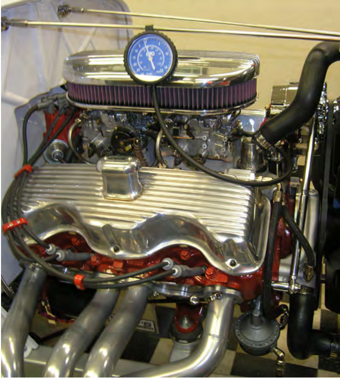
This vacuum gauge is being used to observe what the manifold vacuum is on this 348 Chevy while the automatic transmission is in Drive.
