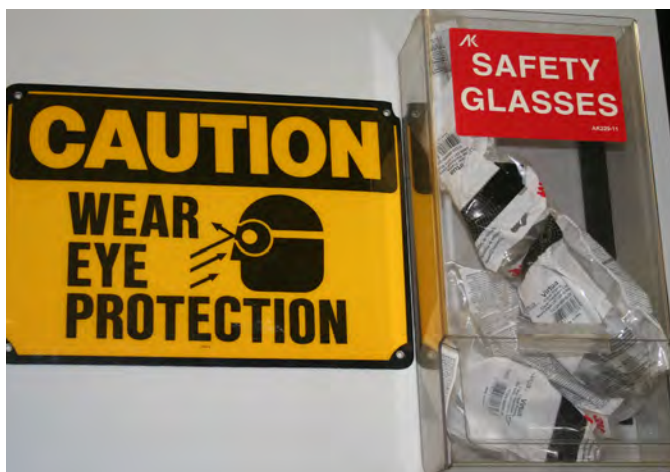
Many shops post signs reminding workers and visitors to wear eye protection. Some shops have safety glasses available. OSHA and local regulations require safety procedures.
