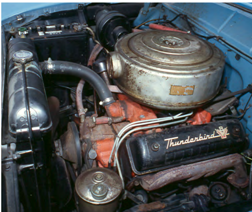
These old Ford Y-Blocks had mushroom lifters. Are you going to put a roller cam in it?
