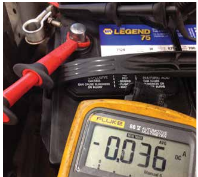
Measuring current draw overnight using MIN/MAX.
