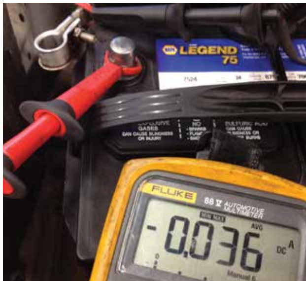
Measuring current draw overnight using MIN/MAX.
