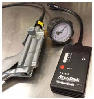
Nissan recommends using an ultrasonic tester and hand-held vacuum pump to find leaks. Vacuum decay (vacuum decreasing over time) indicates that there is a leak. The ultrasonic tester is used to locate the source of the leak.
