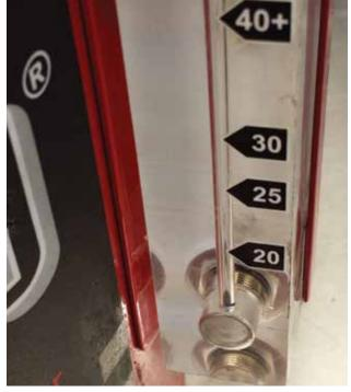
If pressure regulated at 0.5 psi is applied to a sealed EVAP system, the amount of flow in should be equal to the amount of flow lost through the leak. A pressure supply and a flow meter is another way to determine if the EVAP system is leaking.
