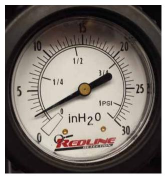
Pressure decay (pressure decreasing over time) is another way of determining if the EVAP system is leaking.
