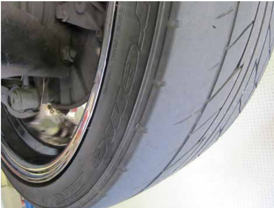
Here you can see tire wear and damage from an oversized wheel -- three inches larger than stock. This W220 also had heavy tie-rod wear/play from the sheer weight of the aftermarket rims.
