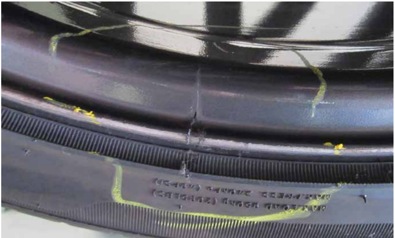
This GL450 has a damaged aftermarket wheel from hitting a pothole. There was not enough sidewall to absorb the impact. Also, this rim's construction is inferior with too much offset
