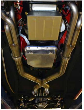
Here's what the entire system looks like, and you have to admit it's impressive. Everything clears, it tucks up nicely under the car (important here in the Midwest where every winter turns our roads into tank trap testing facilities), and access to normal service items is unimpeded.
