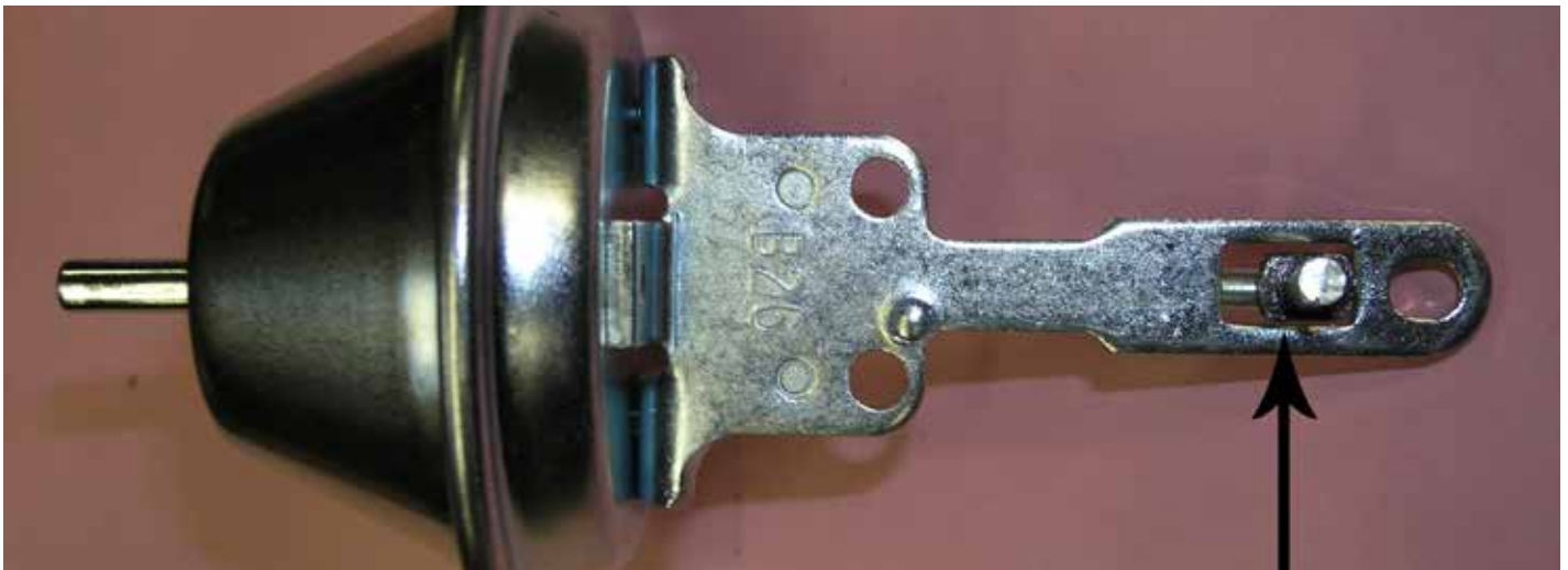
The arrow in this picture points to the bushing that was used to limit the vacuum advance to 10 degrees of spark timing.
